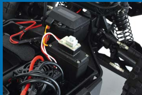
Even the switch on the Reedy SC600-BL is waterproof
