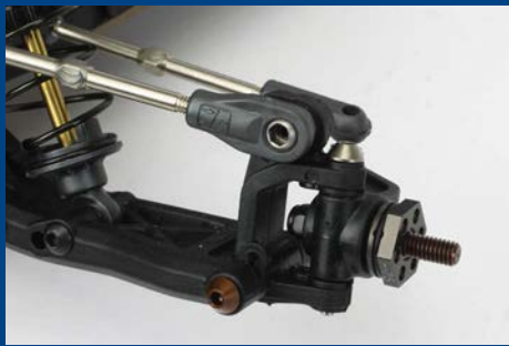
The design of the caster block and steering arm is incredibly compact
