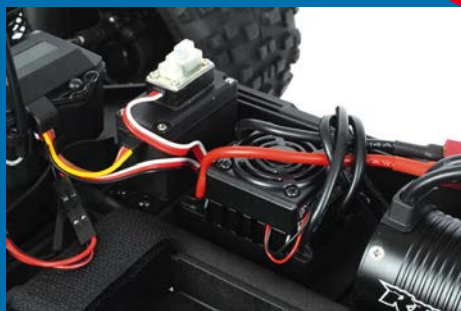
To match the Reedy motor is a brushless speed controller in the form of the SC600-BL
