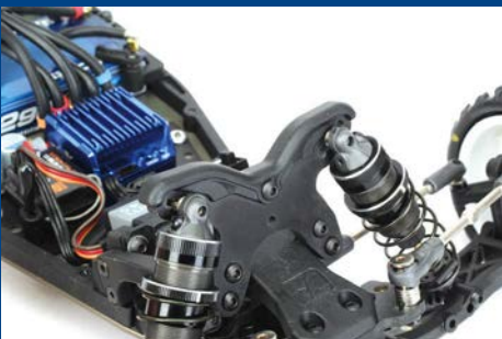
The LD2 comes with "S2" material 4mm thick shock tower mounts
