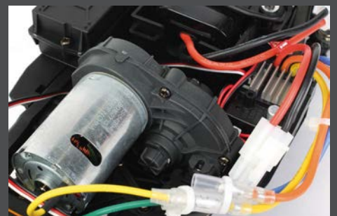
Due to its use, the plastic used for the gearbox is of a grey colour and a different spec compared to the chassis
