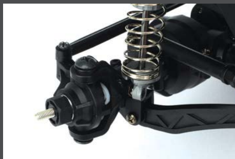
The CC-02 comes with plain bushes as standard, but an upgrade to bearings is cheap to do
