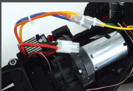
A Tamiya connector for the battery whilst only two of the three motor bullet connections are used
