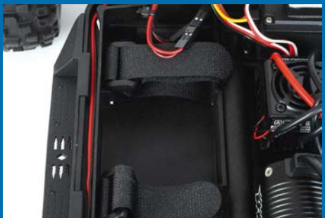
A pair of Velcro straps are used to retain the LiPo in the battery compartment
