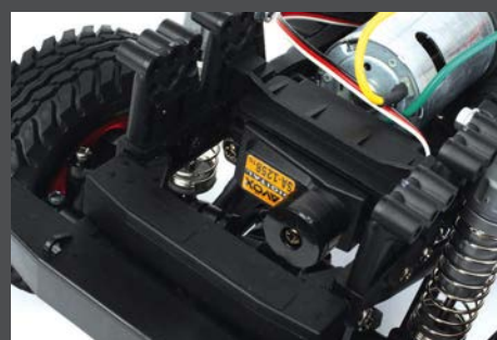
We opted for a more powerful Savox servo for steering duties in the form of an SA-1258TG Digital example
