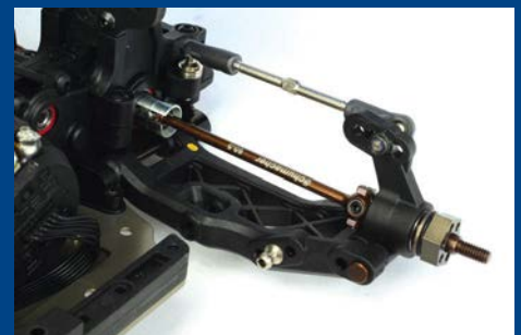
The new 90-degree phased steel CVD driveshaft design
