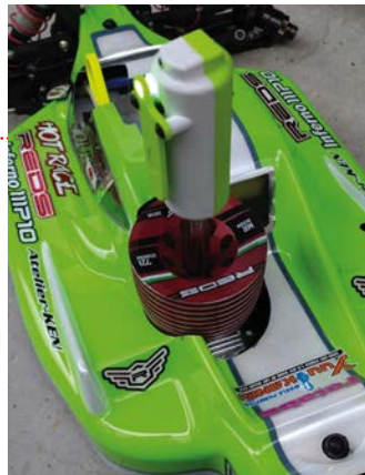
When a plug broke, an LED doesn't light up
