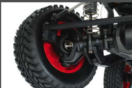
The silver-coloured linkage from the servo connects to the right steering arm with a longer moulding to the left side
