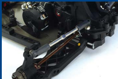
One area that might be a weakness are the turnbuckles as there is only a small amount of thread in the ball cup
