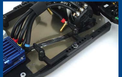
Machined grooves in the chassis keeps the sensor lead out of harm's way
