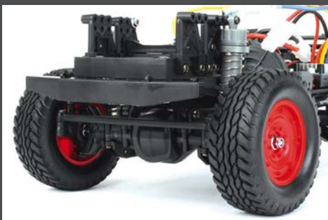
The steering arrangement uses a long moulding to connect the left and right arms
