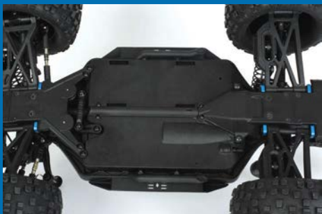
The chassis sits up higher than the front and rear gearboxes to maximise clearance
