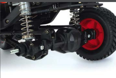
The rear axle setup features a diff in the centre. This is better in general use compared to a locked arrangement
