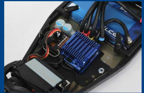
We chose a proven package of Spektrum servo and receiver, with LRP power
