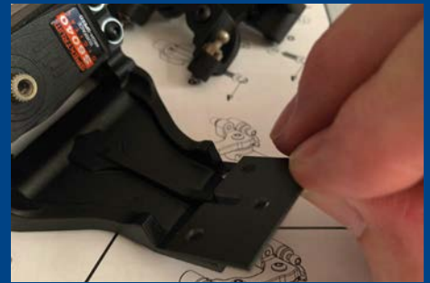
The bulkhead height can be increased using the shim that also alters the pivot position of the front wishbones
