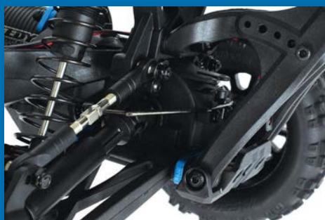
Telescopic-style mouted driveshafts feature front and rear
