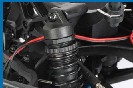
Threaded collars on the shock absorbers are used to set the ride height
