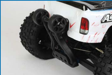
The wheelie bar is tucked neatly out of the way when it is not required
