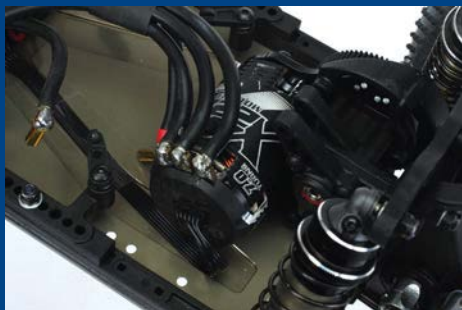
A 7.0T motor is a popular choice in 2WD and we went with an LRP X22 example
