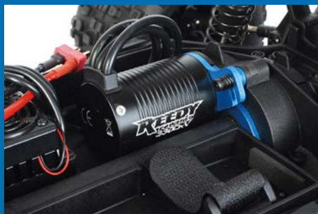
The motor is a Reedy 3300kV brushless model and offered plenty of power
