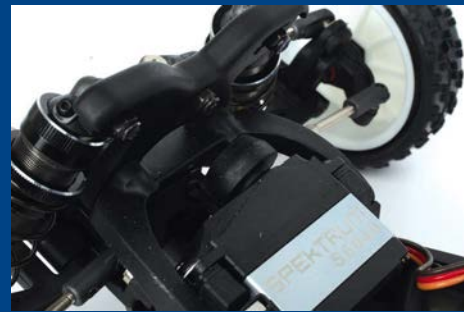
It is interesting to see that the LD2 now comes with a servo saver in the box
