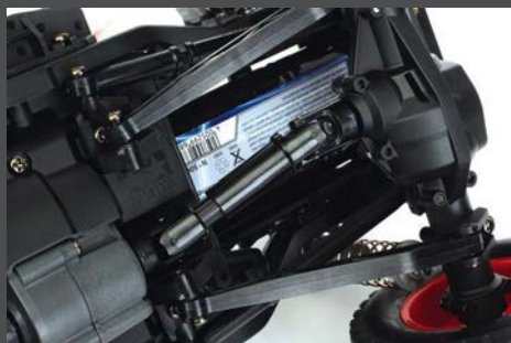
Telescopic moulded driveshafts ensure permanent 4WD is retained even during extreme chassis articulation
