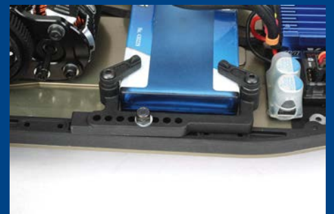
The new LiPo-retaining mouldings can be seen here as well as the adjustment for the battery position
