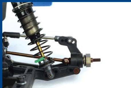
Inner and outer pivot positions on the rear hub and wishbone
