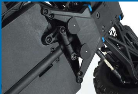
The steering linkage is shielded as the servo sits up high in the chassis
