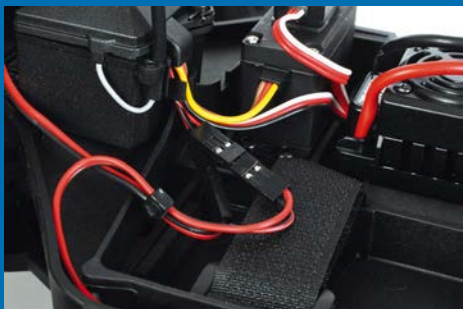
All the wires for the LEDs and from the speed controller are neatly inserted into the receiver box
