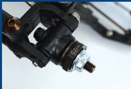
An O-ring ensures the pin stays in place through the front axle
