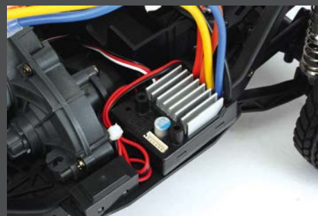
The included speed controller, a Tamiya TBLE-04S, can be used with both brushed and brushless motors
