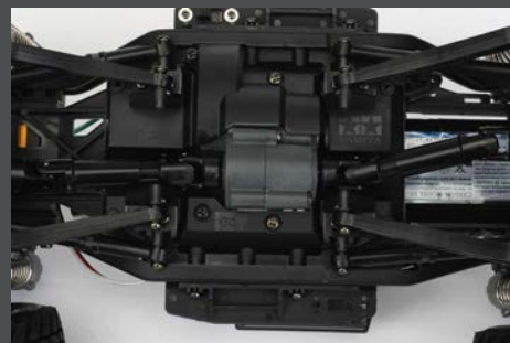
The gearbox moulded uses a different spec of plastic compared to the chassis
