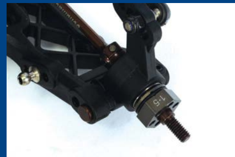
The rear hex width is clearly marked
