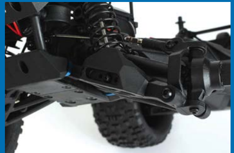
Guards in front of the shock absorber lower mounting
