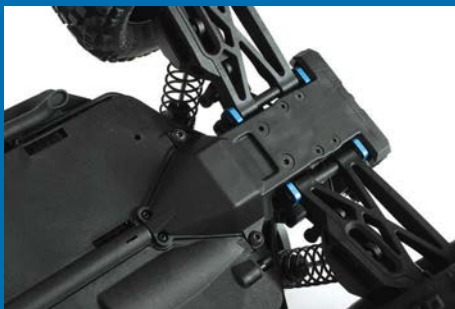
An angled moulding ensures the rear of the chassis glides over obstacles rather than getting hung up
