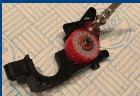
The machined idler gear, which used to be an option, is stronger and quieter, and now comes as standard
