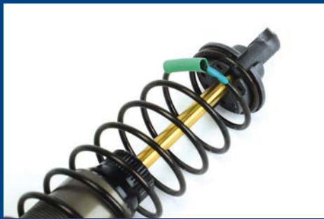
A bit of paint and heatshrink indicates the green spring rate
