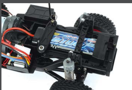
The battery compartment is plentiful so we would add a little foam to fill the space and add some protection
