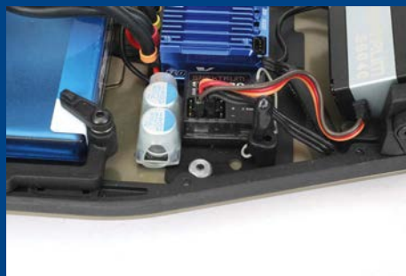
The speed controller and receiver are mounted to a removable GRP radio plate
