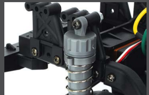
On each corner is a moulded oil-filled shock absorber
