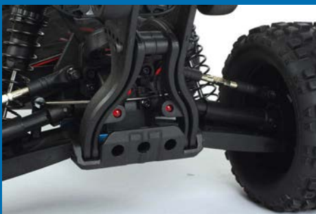
Here you can see the rear anti-roll bar that helps when the truck corners at speed
