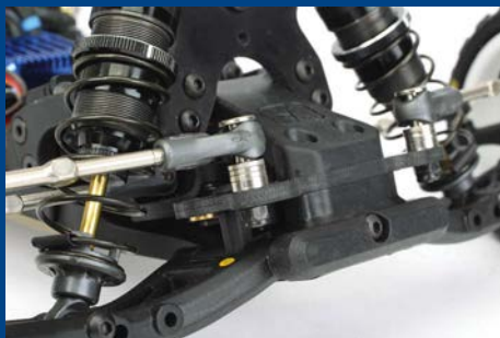
The kit setup uses lots of washers under the inner pivot
