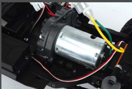
Like many of its other kits, Tamiya has chosen to equip this Unimog with a Mabuchi 540-size silver can brushed motor
