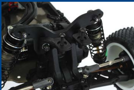
The mounts are very narrow and the wing sits low off the rear tower
