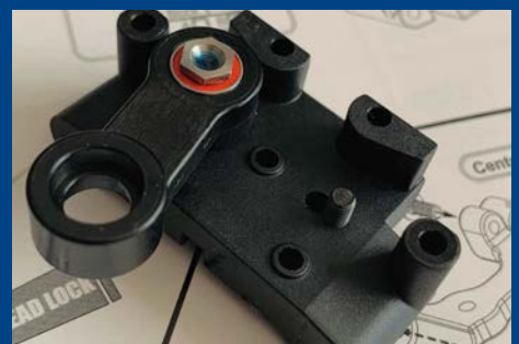
There is choice of an inner and outer hole for the steering arm posts to secure to that alters the Ackermann
