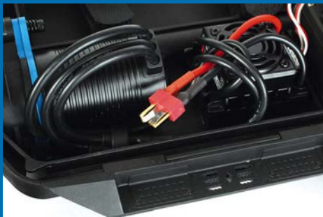
A Deans connector is an ideal choice for its popularity and simplicity
