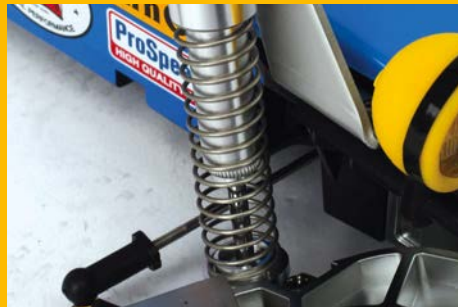
The front springs are full length and are supplied without any spacers to alter the ride height
