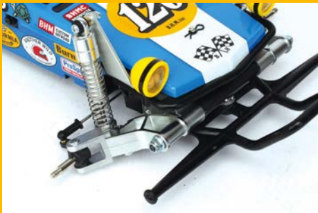
The wide plastic bumper offers protection across the whole of the front suspension
