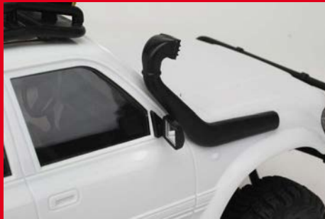
The snorkel fitted to the injection-moulded hard body adds to the scale looks. You can also see the detailed interior
