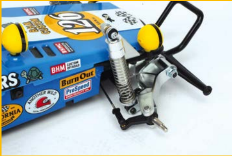
The front shocks are oil filled and locate on the rear of the front suspension arm
