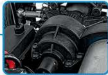
A sealed center driveline keeps dirt and debris out—along with bits of tire rubber—for smooth and reliable power delivery
