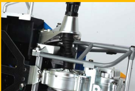
Rubber boots cover the whole of the rear driveshaft
