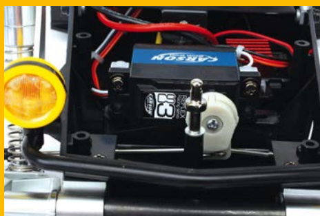
A Carson servo was installed to match the rest of the electrical components
