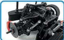
For better handling, A-arm front and rear independent suspension keeps the Hoonitruck under control during the wildest of driving conditions
