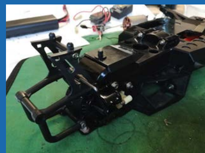
The rear view showing locked out steering rack (in white) for optional 4-wheel steering
