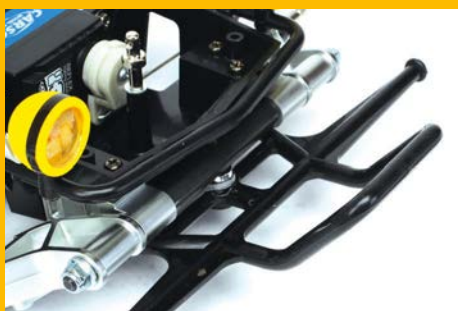
A single shaft passes through both front arms to allow them to pivot
