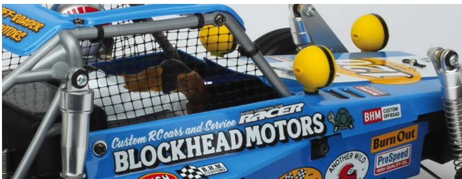
The body panels have been designed to look like they are bolted onto the roll cage assembly
