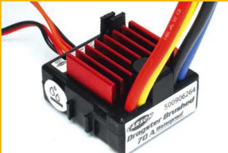
Our sample included a Carson Dragster Brushed 70A Waterproof speed controller
