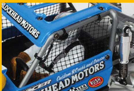
The body panels have been designed to look like they are bolted onto the roll cage assembly
