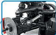
Active rear suspension allows the amount of toe change to be adjusted through the suspension cycle, increasing or decreasing rear grip
