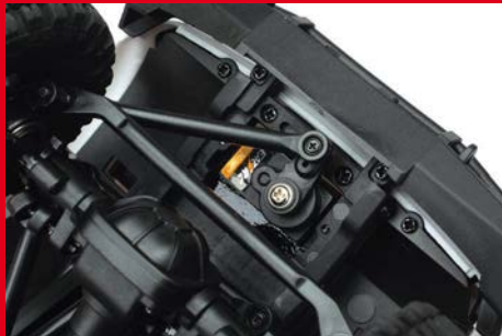
Facing down is the chassis-mounted servo from Eazy RC
