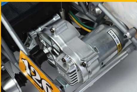
Tamiya moulded the gearbox casing in an aluminium-coloured plastic that is very realistic
