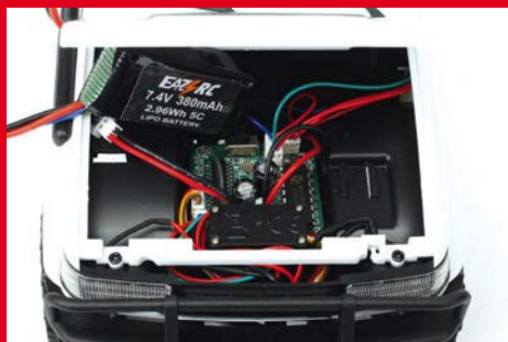
The Eazy RC LiPo battery sits behind the combined speed controller/receiver unit
