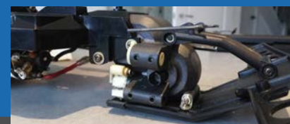
The gearbox assembled onto the car. The white cam adjuster is for altering the camber at the wheel
