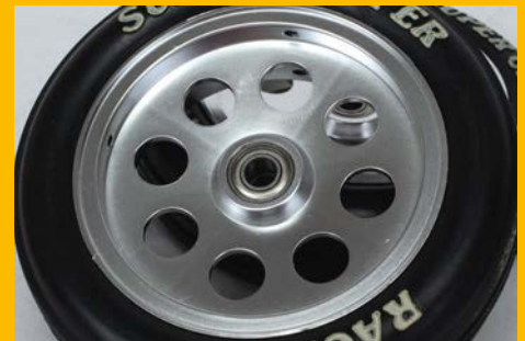
Optional bearings replaced the stock bushings in the front wheels
