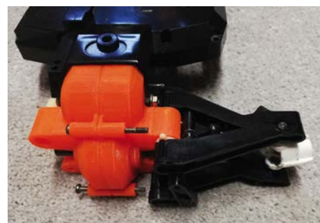
The trial installation of the gearbox casing to confirm fit
