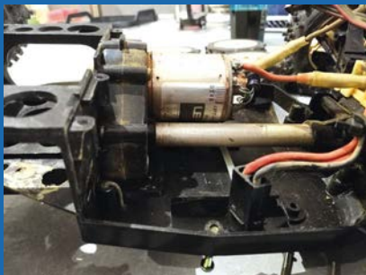
Inside the car as it had arrived, complete with Kyosho LeMans motor and Sanwa speed controller (not shown)
