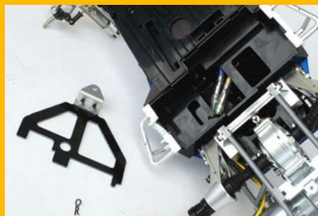
A body clip secures the battery strap in position for easy and quick access
