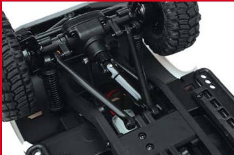
The Patriot comes with a link-type front suspension and shaft-drive transmission
