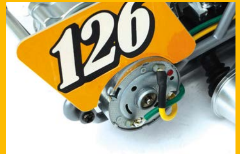
The rear number board is shaped to go around the brushed motor
