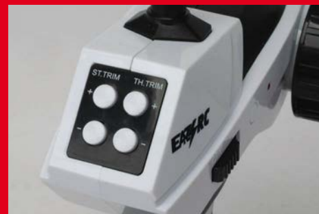
Buttons on the 2.4GHz steering wheel transmitter alter the trim settings
