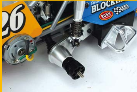
At the rear of the Wild One the design uses a trailing arm setup
