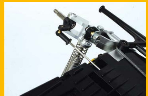
The ball ends and linkages are very thin compared to modern setups, but they are a period design
