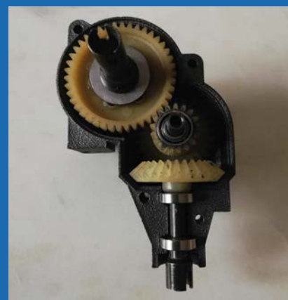
MJF-printed gearbox moulding going together for actual running
