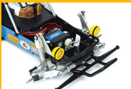
With the body removed it is easier to see how the suspension mounts to the chassis
