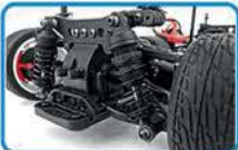
Threaded oil-filled shocks smooth out the bumps when ripping down the tarmac and shredding tires
