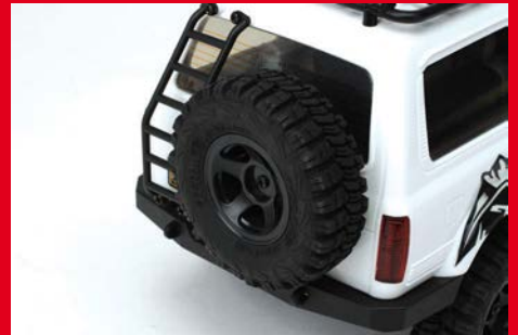
Bolted to the rear door is a useable M/T tyre mounted to a 1-inch internal beadlock wheel
