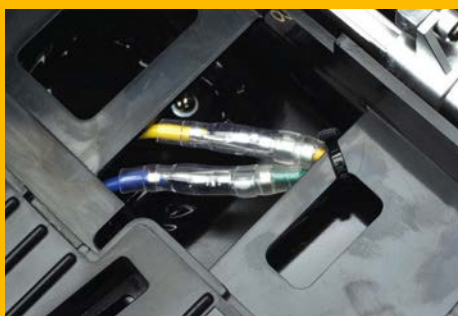
The bullet connectors for the motor are tucked away and out of sight
