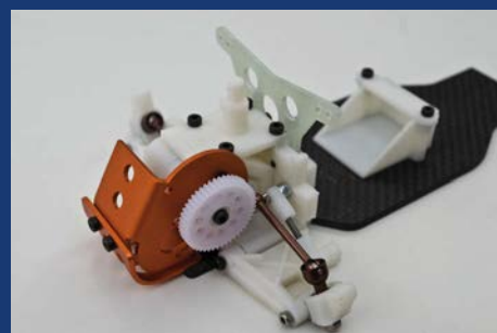
With the gearbox bolted into the chassis
