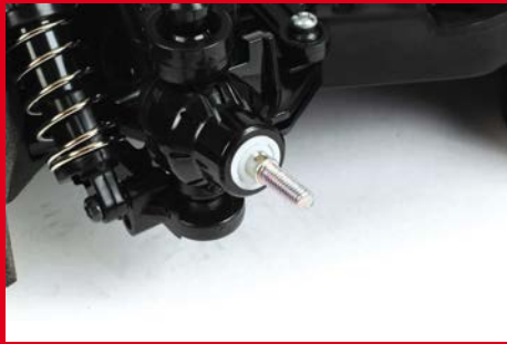
White plastic bushes come as standard and feature throughout the transmission
