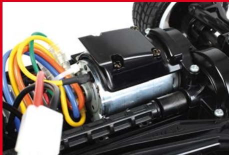
A moulding above the motor directs airflow onto the Mabuchi 540-size motor
