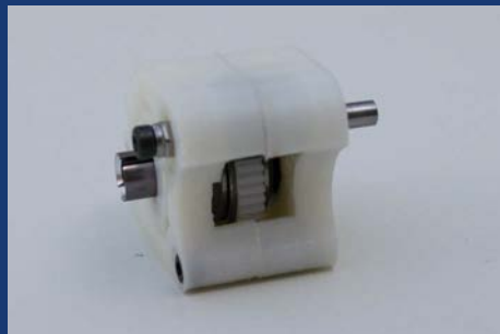
The ball diff gear can be seen through a gap in the casings
