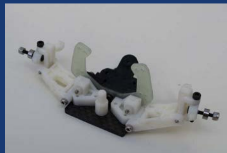
The nose plate supports the front suspension with the body post and shock tower in place
