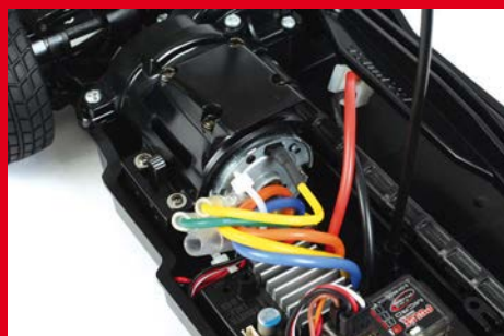
A cable tie keeps the excess length of wires neat and tidy
