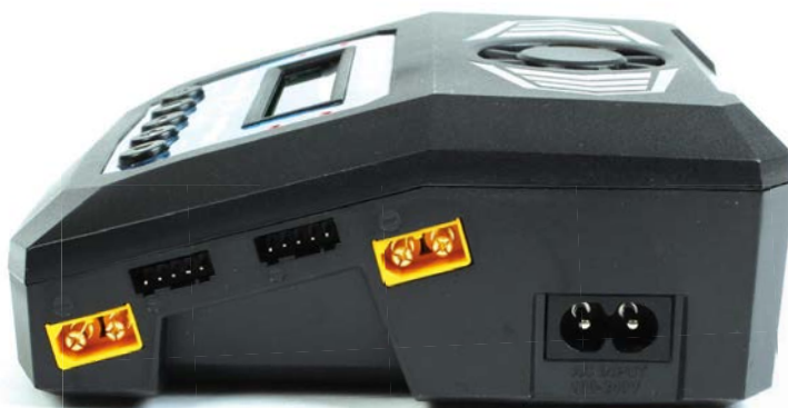
The charger can be used off the mains (AC) or from a suitable DC power supply
