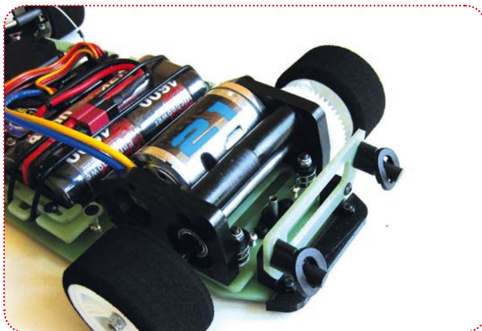
Horizontal body posts makes the hatchback body shell easier to mount
