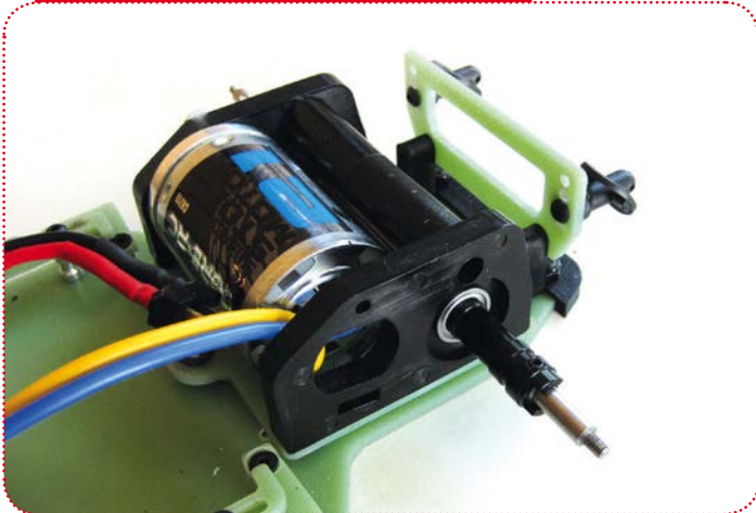
Despite its low cost the VRX HR3 features bearings throughout
