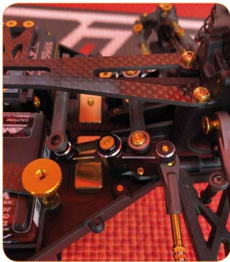
Alloy steering components over flex-free operation with the best driver feedback
