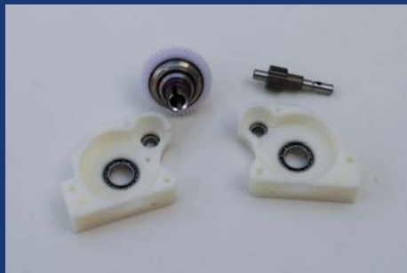
The gearbox has just two gears with the layshaft and diff gear
