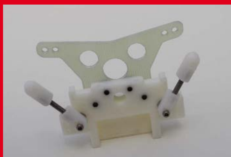
The rear bulkhead is secured to a natural-coloured shock tower
