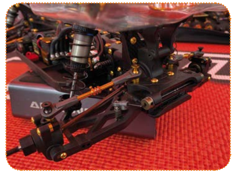
Vertical ball studs at the rear add to the huge tuning potential of the SRX-4 Gen3
