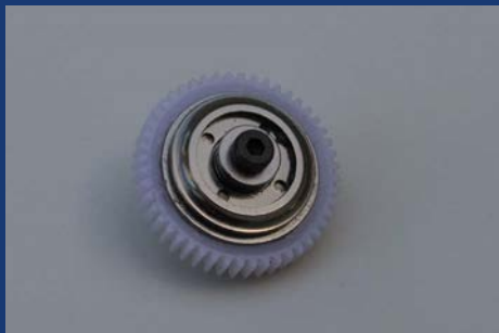
As it's period correct, the kit comes with a ball differential
