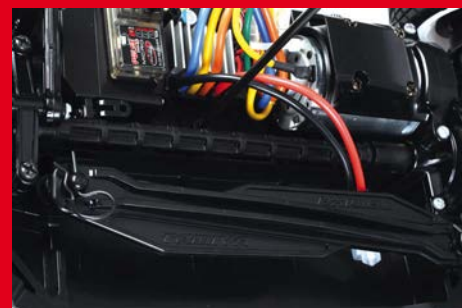
Down the centre runs the moulded plastic propshaft linking the drive front to rear
