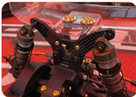
Both the front and rear shock towers are machined out of 4mm thick carbon fibre
