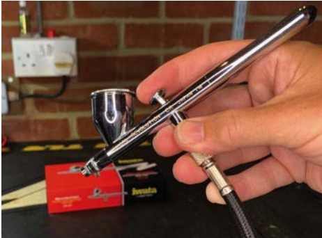
You hold an airbrush like a pencil, pushing down and pulling back to control the air and paint respectively
