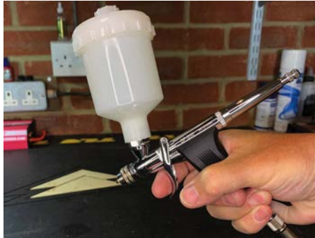
The Sparmax GP-850 is a single-action airbrush that uses a simple trigger to operate
