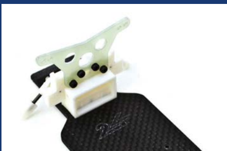
The rear bulkhead assembly is screwed onto the NRC-24 carbon fibre chassis
