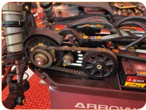
A side belt transfers drive from the rear gearbox forwards
