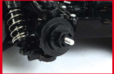
The hex moulding incorporates a dummy brake disc
