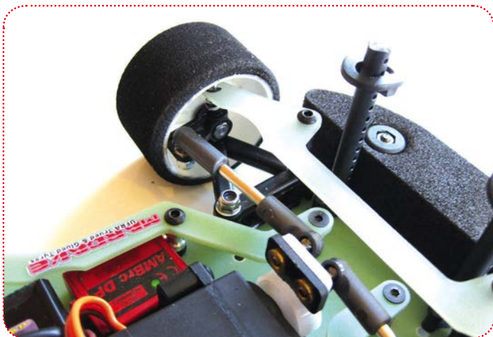
The optional camber strap strengthens the front suspension. The body posts have adjustable height which is very useful
