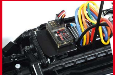
This tiny 2.4GHz receiver sits on top of the steering servo
