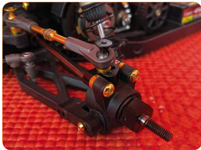
The amount of roll centre options at the rear hub is incredible
