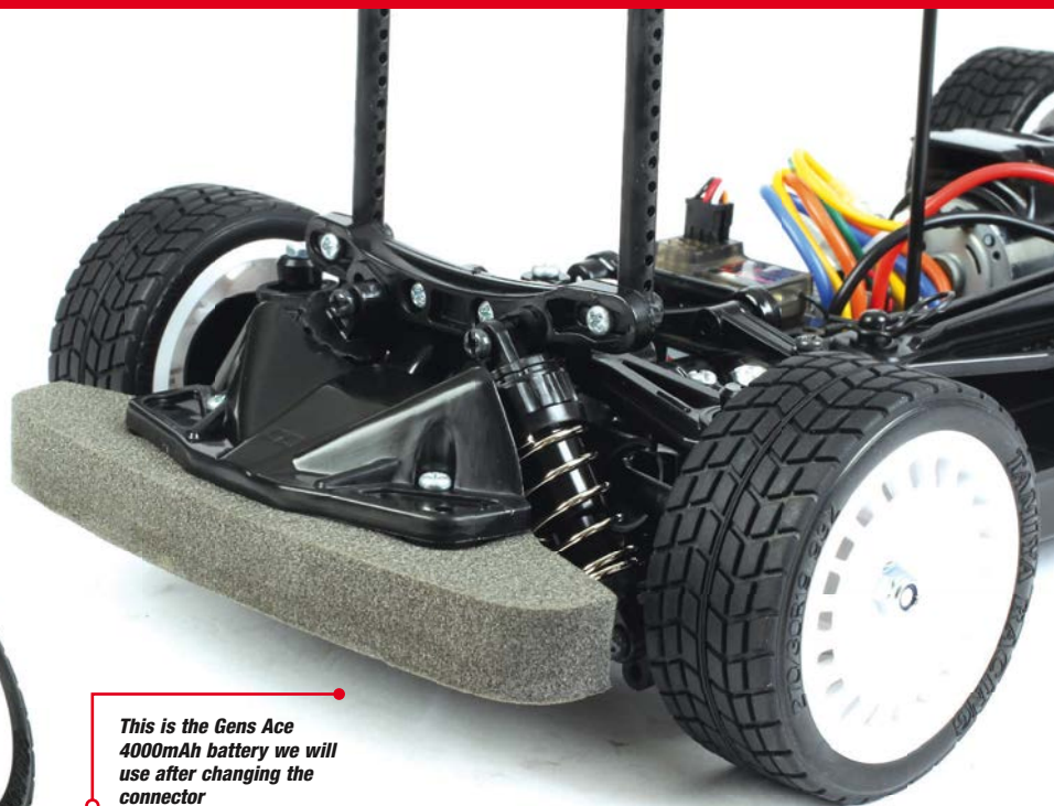
A moulding above the motor directs airflow onto the Mabuchi 540-size motor
