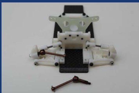
The metal rear driveshafts can now be inserted into the rear hubs
