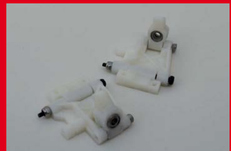
The rear suspension components start to be put together
