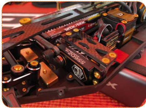
Note the additional weights that bolt to the chassis into designated positions
