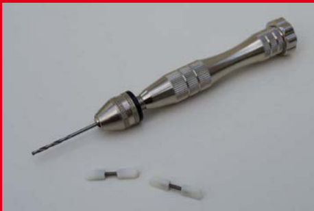
A pin drill is an essential tool to have. It is the sort of thing used to drill out 1:10-scale pistons
