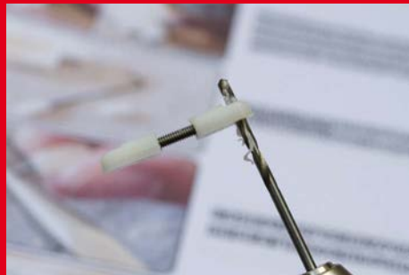
The moulded ball joints are drilled out...
