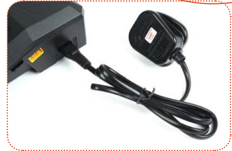
You get a 240 AC mains power cord with the charger but it can also accept an input via a power supply
