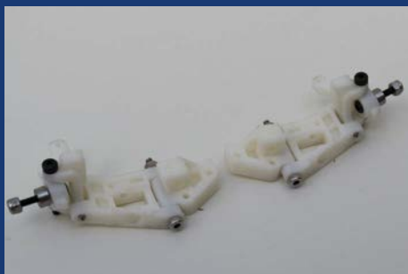
The front suspension units ready to bolt to the nose plate
