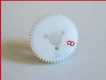
The hot rod uses a 48-tooth, 32DP spur gear - the same as all the original 1:12-scale cars
