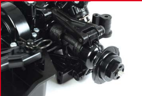
The front and rear driveshafts, like the prop are also moulded plastic
