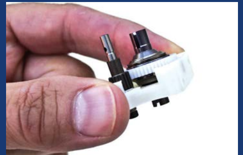
The layshaft and diff are supported by bearings inside the casing
