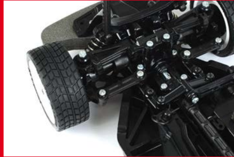
The TT-02 is a quick and easy build aided by moulded linkages front and rear
