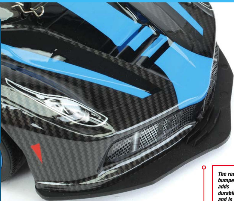
Mouldings in the bumper help to support the front of the body
