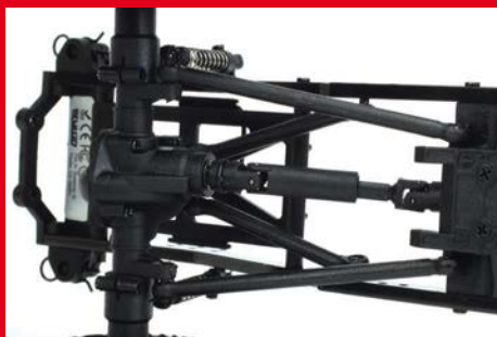
The front and rear axles feature locked differentials for the best traction
