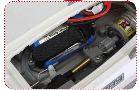
The brass-coloured propshaft is kept clear of cables and other parts that could rub
