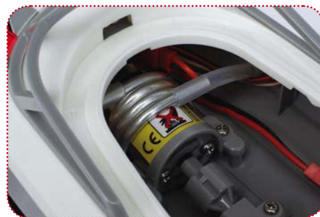
Water is passed around the outside of the motor to aid cooling as there is no airflow inside the hull
