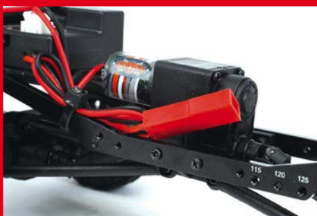
With little load on the components a traditional receiver-type connector is used on the battery
