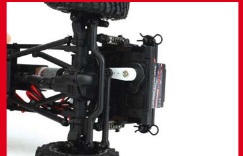
A horn connects the RC4WD Micro Twister servo to the front wheels
