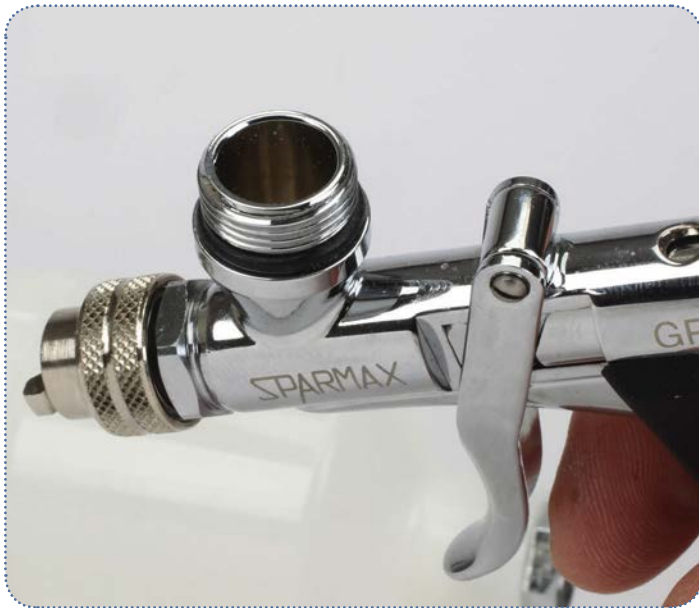
The plastic paint cup screws onto the body and is sealed by an O-ring
