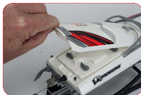
The magnetic top cover hides a more substantial lower one that has a seal to prevent water ingress
