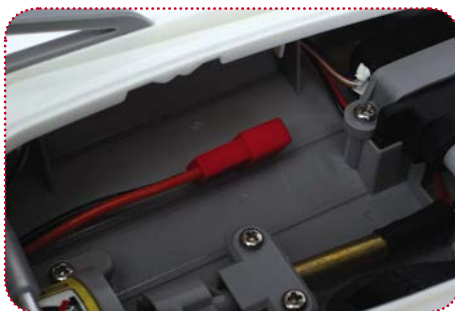
As there isn't too much load, the battery connector is fairly light weight
