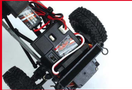
The 1:24-scale model uses a combined speed controller and receiver unit
