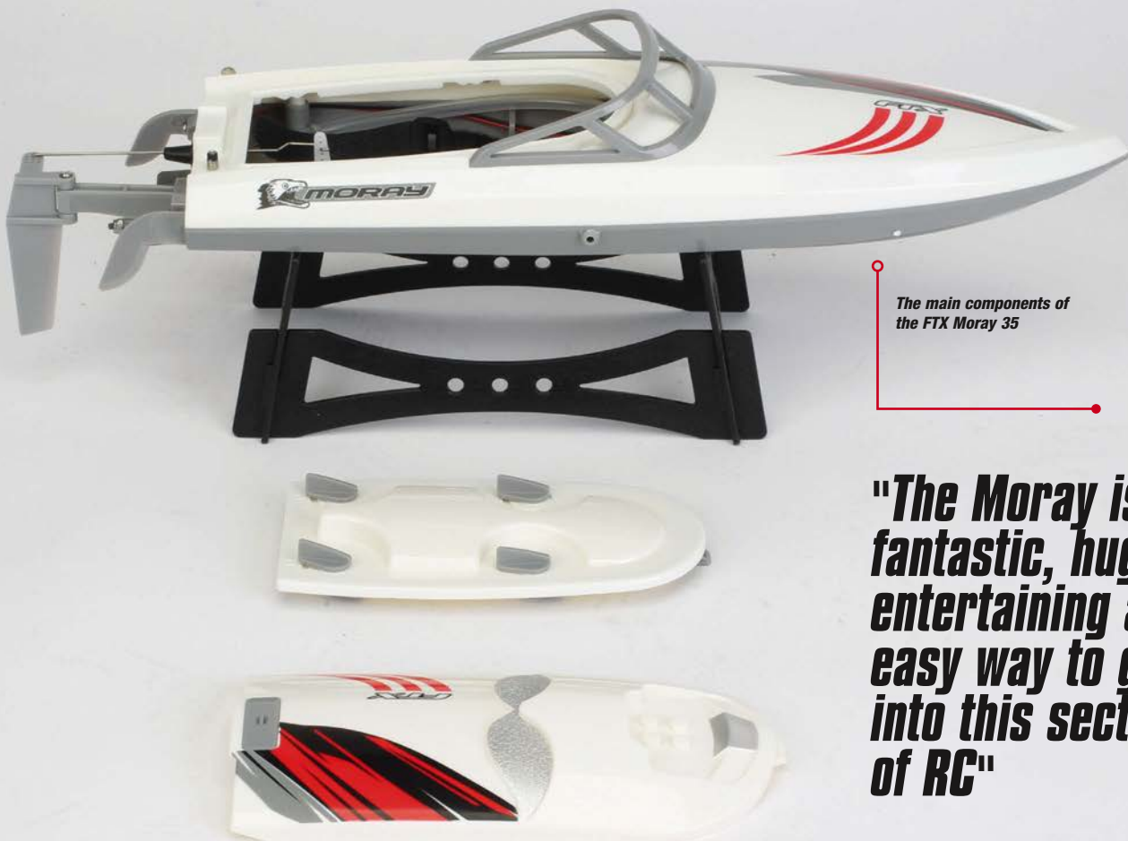
Four of these latches ensure the cover sits tight against the seal to the hull
