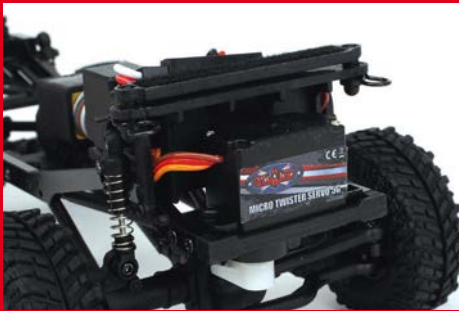
The steering servo sits above the front axle to add weight and therefore traction
