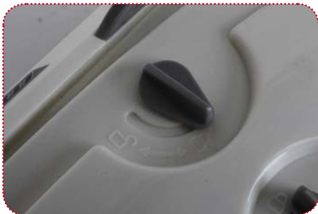
Four of these latches ensure the cover sits tight against the seal to the hull
