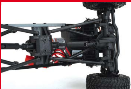
Moulded telescopic driveshafts are used for the centre drivetrain
