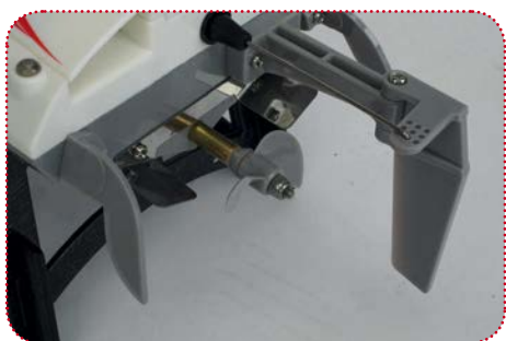
The prop can be easily changed if damaged as its held in place by a nut
