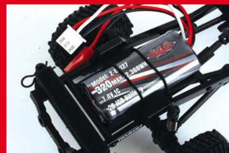
The tiny 7.4V LiPo battery is rated at 320mAh and is held in place by O-rings
