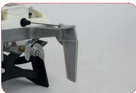
The chunky rudder is a moulded item
