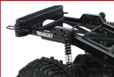
The chassis rails are machined from aluminium and have the usual RC4WD attention to detail
