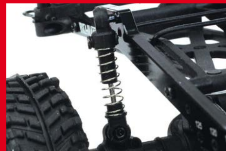
The suspension movement is controlled by a simple spring setup
