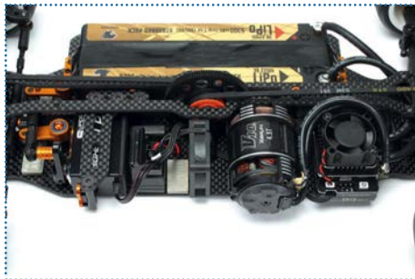
A Hudy 10g weight is used to balance the chassis from side-to-side
