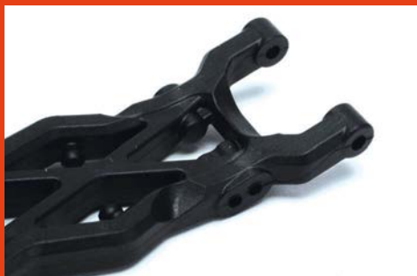
The symmetrical rear wishbones can be flipped to set the choice of three lower shock mounting positions. There are two holes on one side and one on the other
