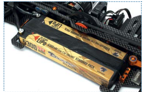
Tape is used to secure the LiPo in place
