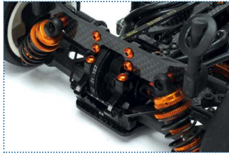
At the rear its a softer 1.2mm anti-roll bar and less droop than the front
