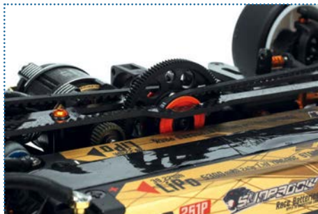
Xray's own 64dp spur and pinions are used
