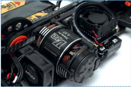
The Hobbywing V10 4.5T motor is kept cool with a dedicated fan in front of it
