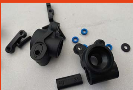
The new rear hub design features a modular vertical ball stud camber link mount and uses inserts to adjust the pin height and toe in
