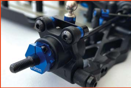
Wider wishbones mean narrower 5mm offset hexes are used front and rear
