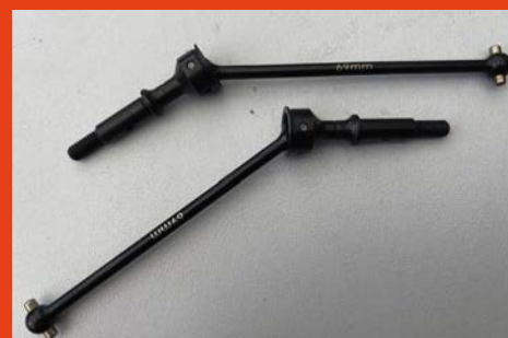
As the B6.2 uses a long wishbone, the driveshaft is of a matching length at 69mm to reduce the bone plunge and minimise friction at the drive pin
