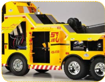
The hatches allow for handy internal access
