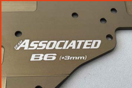
The lightweight 7075-T6 hard anodised chassis that comes with the B6.2 is 3mm longer than the one supplied with the dirt-spec model
