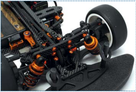
Olly's starting setup features progressive springs up front and a 1.4mm anti-roll bar
