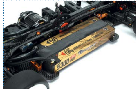
This 5300mAh capacity LiPo from Sunpadow is one of their low centre of gravity packs
