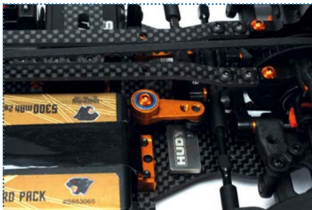
The T4'20 is underweight as standard so Oilly sometimes places the ballast at the front to make the car easy to drive to it forward for an 'easier' car.
