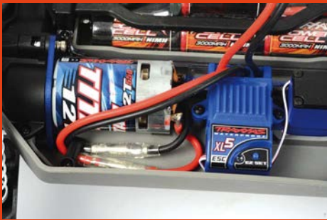
The Stampede 4x4 Kit is powered by a brushed setup with Traxxas's own motor and speed controller included
