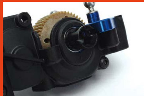
It was only a minor issue but we think that the moulded diff inserts caused a tight spot in our transmission. Two different inserts allow four diff heights to be selected
