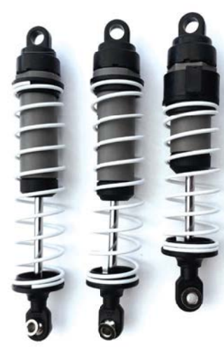
The long travel oil-filled Ultra shocks were super smooth and worked very well in testing
