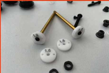
We marked up the pistons sizes for clarity using a permanent marker
