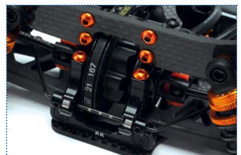
On carpet the team use around 5000cst oil in the rear diff
