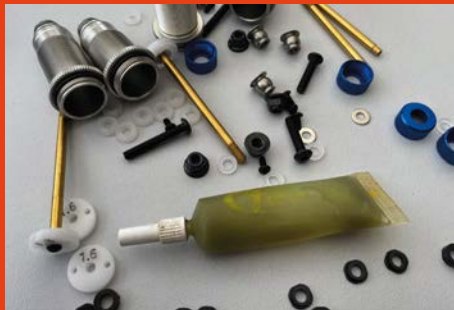
Team Associated FT Green Slime is used to prevent damaging the X-ring seals
