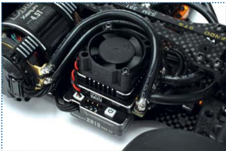
The mid-motor design requires the speed controller to sit at the rear of the chassis
