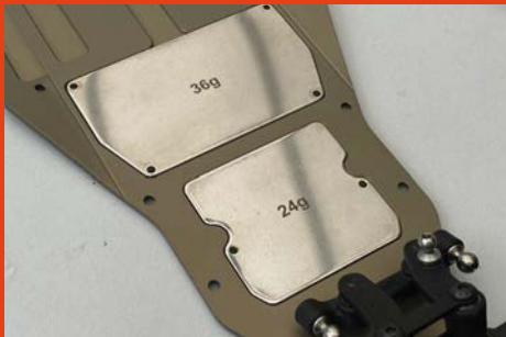
The steel speed controller and servo chassis weights locate in pockets that are machined into the chassis
