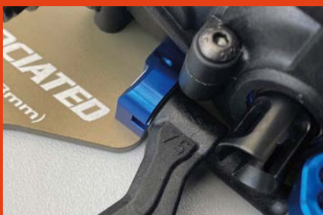
The number indicates that these are the longer of the two B6.2 wishbone and 75mm in length
