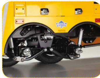
Four wheels and tyres are fitted each side
