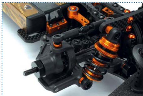
The front shocks use the same pistons and oil, but with a 2.5-2.8lb progressive spring
