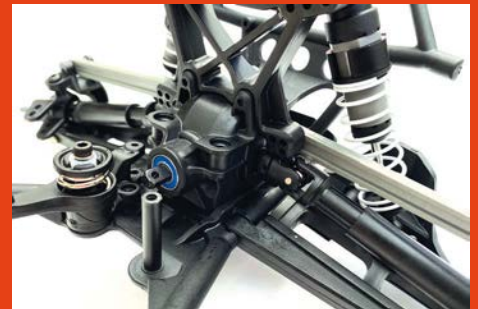
Here you can see the servo saver, blue-shielded bearings, telescopic driveshafts and fixed length upper linkages
