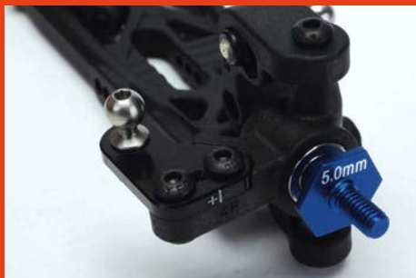
Steel +1 Ackermann steering plates were used on the B6.1D and B6.1DL model and have been carried over to the newest model
