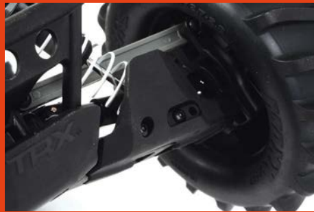
Neat guards protect the vulnerable lower shock mounting on the wishbone
