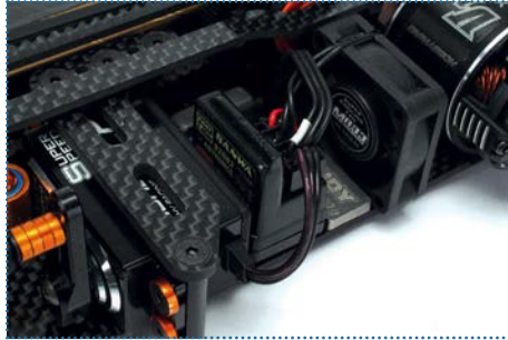
A low-profile Highest servo and Sanwa antenna-less receiver keep things neat
