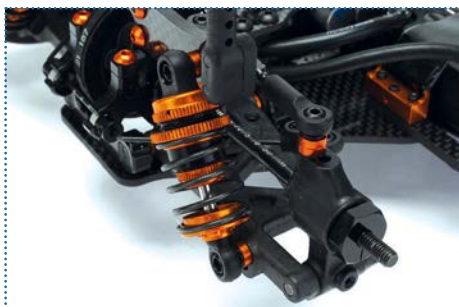
Inside the rear shocks are 1.1mm pistons, 450cst oil and 2.6lb rated springs
