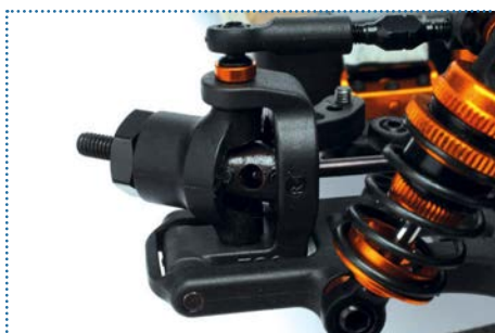
The T4'20 comes with double-joint front driveshafts as standard
