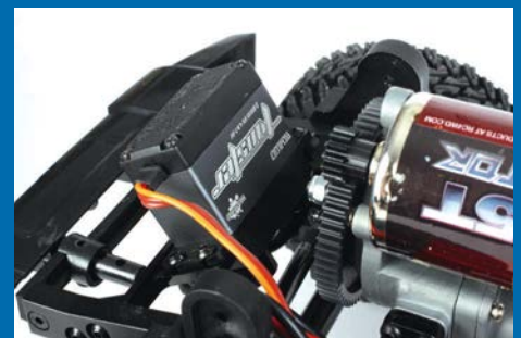
An RC4WD Twister digital high-torque servo steers the front wheels
