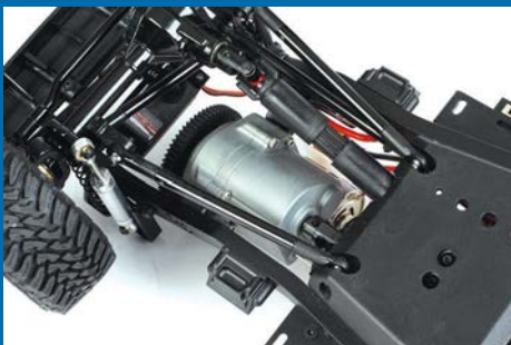
The Cross Country adopts a 3-link front setup with a Panhard rod...
