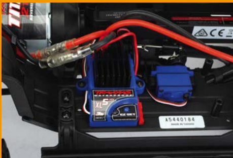
The XL-5 HV speed controller includes dedicated Trail and Crawl profiles
