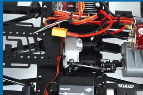
The separate Hammer transfer case is located in the centre of the chassis
