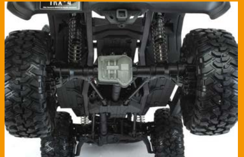
In order to achieve the same pumpkin clearance with straight axles, the tyres would have to be much taller
