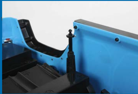
These posts are secured to the body and then click into place in the chassis
