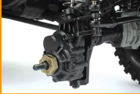
Portal axles lift the truck at the wheels for increased ground clearance
