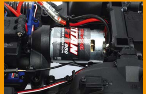
The Titan 21T 550 motor has been chosen because of the huge amount of torque it can deliver
