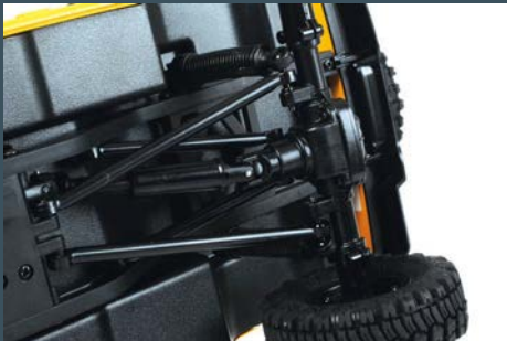
The Arizona uses a multi-link suspension setup front and rear
