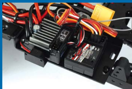
An Outcry III takes care of controlling the speed whilst a 2.4GHz receiver matches the RC4WD transmitter
