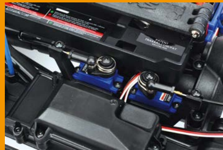
Three small servos operate the front and rear diffs as well as the high/low transmission range selection
