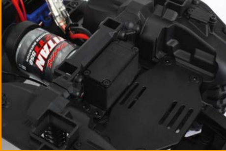
The speed control and servos are waterproof, and the receiver is fully protected by a watertight enclosure
