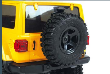
The spare is a full wheel/tyre package and is secured to the rear door
