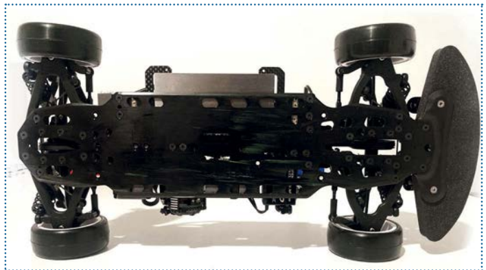
There are three chassis options; 2.2mm graphite or 2.0mm aluminium flex or 2.0mm aluminium solid
