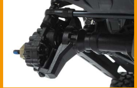
Here you can see how much extra clearance is gained by using a portal axle design
