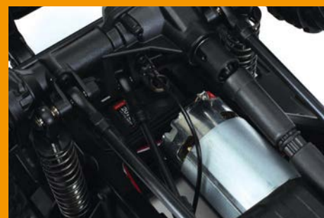
Sleeved cables are used to lock or unlock the diffs front and rear
