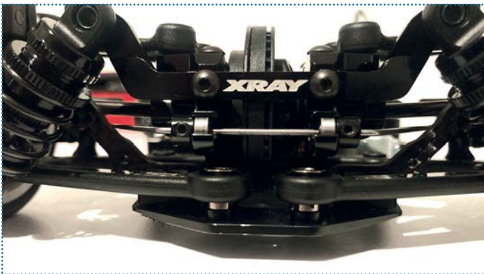
The new CFF suspension arms are mounted via pivot balls directly to the chassis
