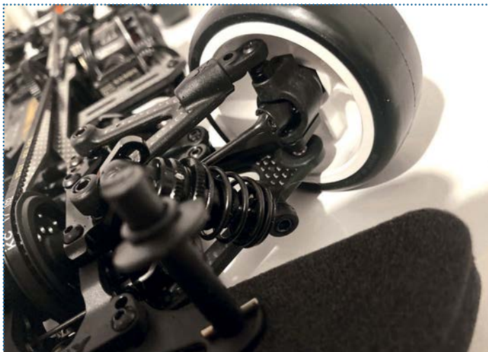
Up front, the standard 58mm driveshafts are recommended and these come in the kit
