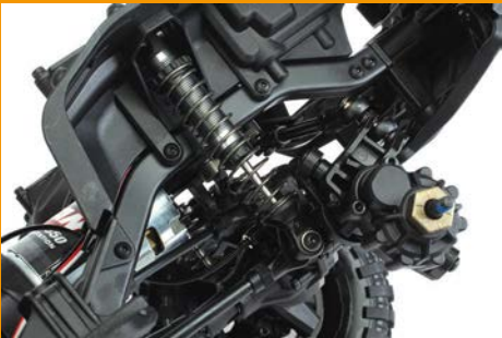
Oil-filled coil-over GTS shocks feature threaded aluminium shock bodies
