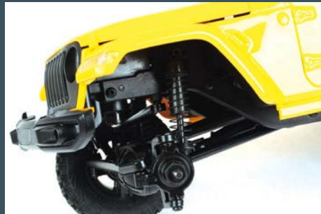
With a wheel removed the shock absorber can be seen along with some of the steering components
