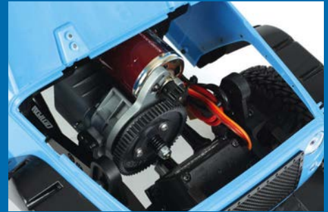
The steering servo sits at the very front of the "engine bay"
