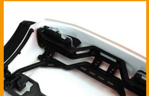
The light buckets are durable mouldings that are secured to the internal frame
