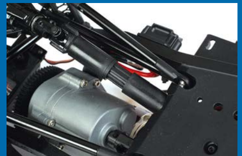
Punisher V2 driveshafts feature heavy-duty universal joints and telescoping nylon bodies
