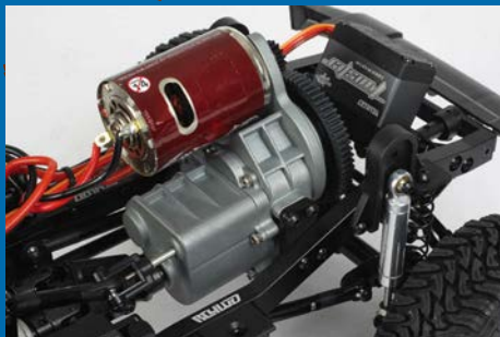
This is the proven R3 2-speed transmission
