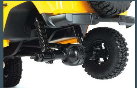
The front and rear axles are both locked for the best traction
