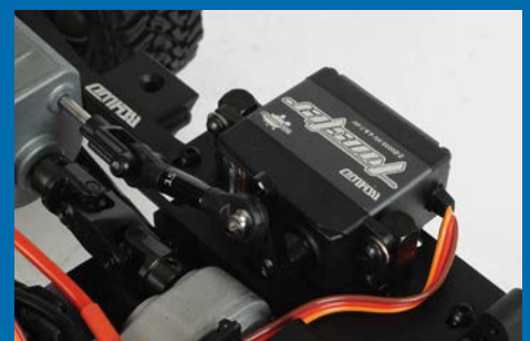
A second RC4WD Twister digital high-torque servo selects either the high or low speed option
