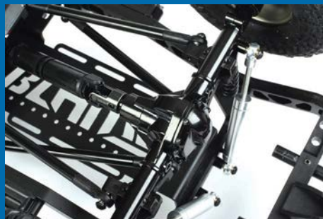
... and a double triangulated 4-link setup at the rear
