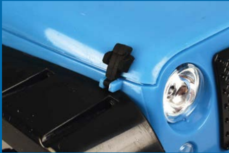
A pair of rubber latches secure the bonnet in place during operation
