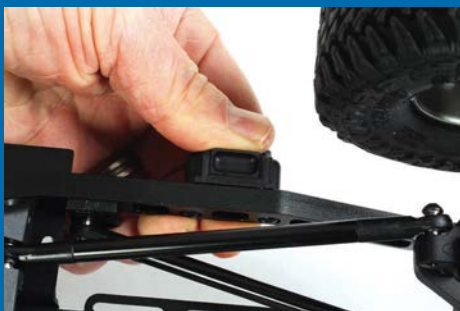
These receptor cavities are attached to the chassis rails and enable you to remove the body
