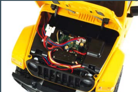
Under the bonnet is the top of the steering servo and the combined speed controller/receiver unit
