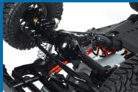
The black pumpkin covers can be removed for ease of re-greasing and maintenance
