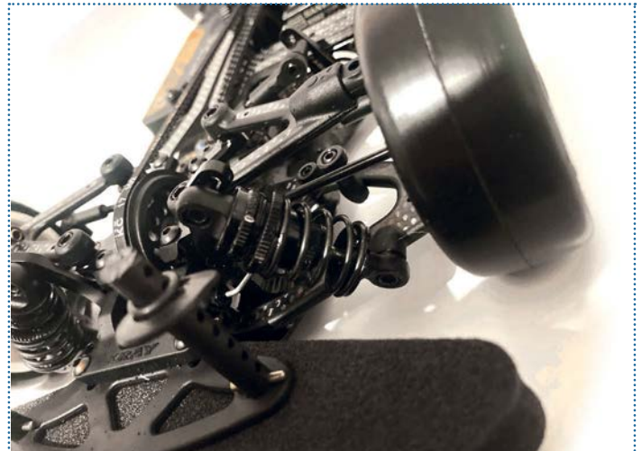
The split aluminium front shock towers are mounted directly to the chassis and have adjustable flex options
