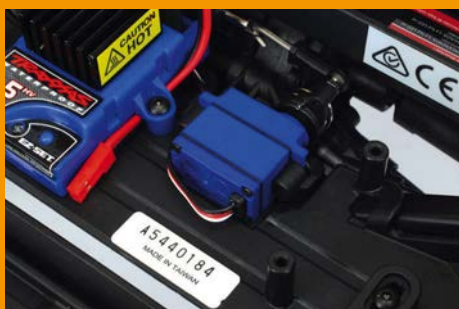
All of the servos, including the three micro-sized ones in blue are fully waterproof
