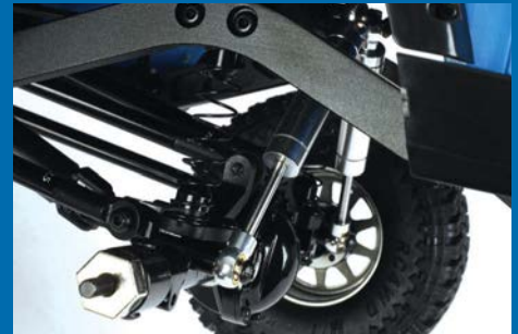
The polished alloy-bodied dampers are combined with separate springs
