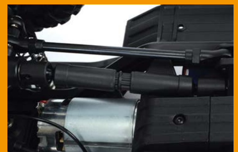
Hardened steel UJs feature on the front and rear driveshafts
