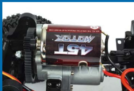
The model comes with an RC4WD-branded 45T brushed motor
