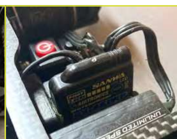
The receiver is very vulnerable due to the many holes for plugs so gets a decent waterproof coating. Note that the Sanwa receiver is marked waterproof
