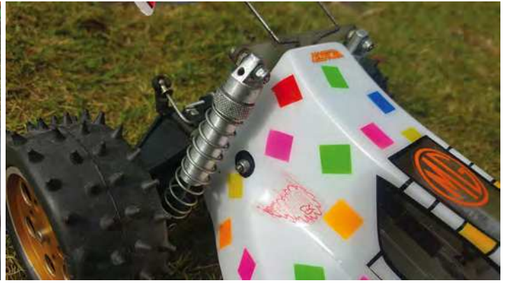
An example of some early Brimod shocks fitted to a Schumacher CAT
