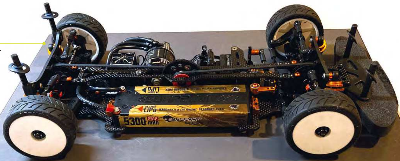
The completed wet car with tyres fitted and battery connected for bench testing
