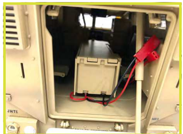
The battery connector extends out of the box and is easily accessible through the opening rear door
