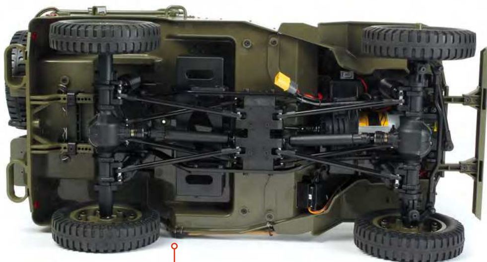
The ladder-frame chassis supports the body-on-frame design, and the suspension that features oil-filled shocks and leaf springs
