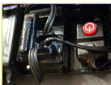
The receiver is very vulnerable due to the many holes for plugs so gets a decent waterproof coating. Note that the Sanwa receiver is marked waterproof
