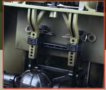
There is some adjustability in the design like here for the body mounting position
