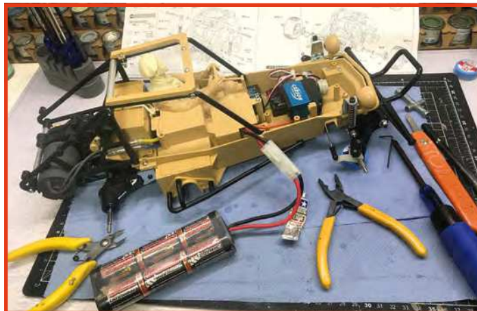
With the figure complete work on the buggy itself could begin. It was straightforward to build thanks to the detailed instruction manual and came together quickly. The only other additions were some metal bearings to replace the plastic bushings that comes as standard in the kit
