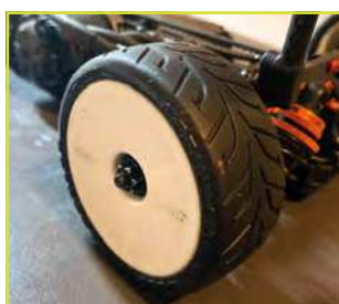
The wet tyre used in the UK is a directional one
