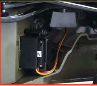
A second smaller servo is fitted to rotate the steering wheel for extra scale detail
