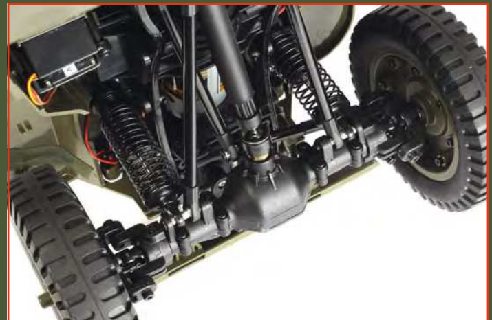
Each axle offers a locked set-up and permanent 4WD
