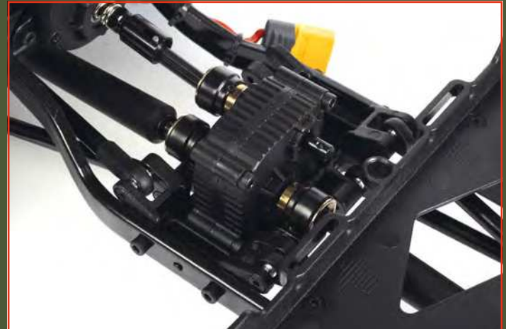
The centrally located transfer box sees drive from the motor come in from the gearbox and then exit towards the front and rear for the all-wheel drive transmission
