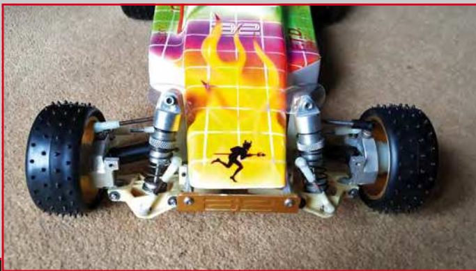
This RC10 4WD Concept has a set of threaded S Type shocks installed all round
