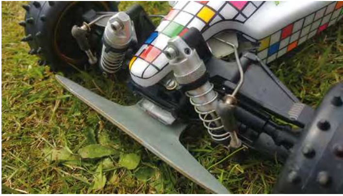
Clip-on spacers are used to set the ride height and there is a bleed screw located in the cap
