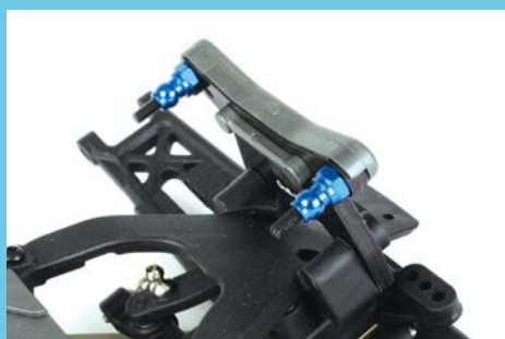
Here you can see how a second moulding on the back of the tower holds the protector in position
