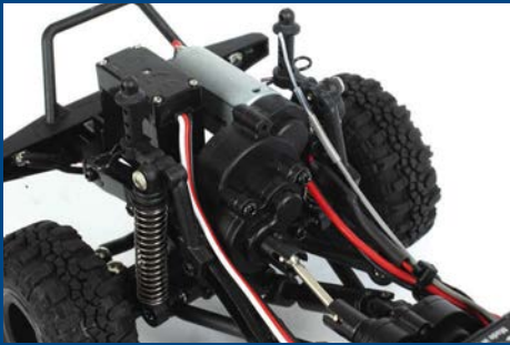
There is lots of weight located over the front axles for the best off-road performance
