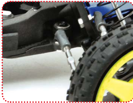
For clearance traditional ball studs are found on the inside pivots for the camber and steering linkages
