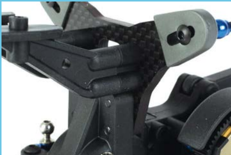
The rear wing mounts are less prone to bending as they use more material. Note the hole for an optional brace
