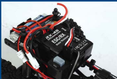
The Team Associated RX-45 is a combined speed controller and receiver unit
