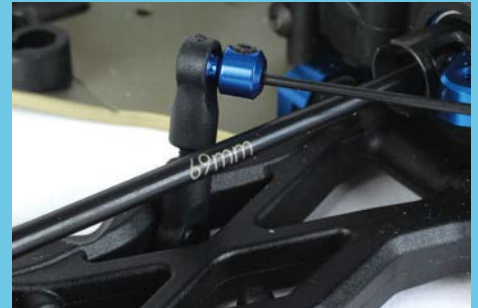
The 69mm long CVA driveshafts mean reduced dogbone plunge that also minimise the friction at the drive pin
