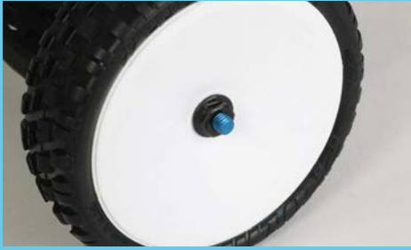
The new low-profile serrated black wheel nuts contrast nicely against the blue axles and white rims
