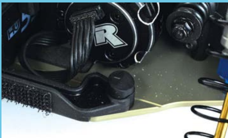
You can fit the fan mount moulding which is included but we went for the blanking option
