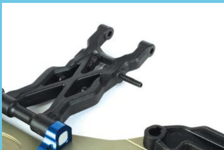
In order to achieve three different lower shock mount positions the rear wishbones can be swapped side to side
