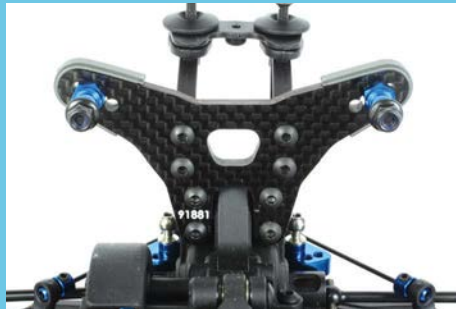
The carbon fibre rear shock tower is marked up with the part number and has revised locations
