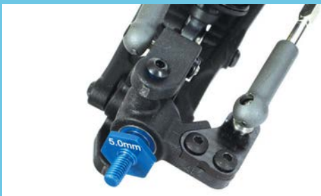
New carbon fibre +1 steering arms replace the older metal versions
