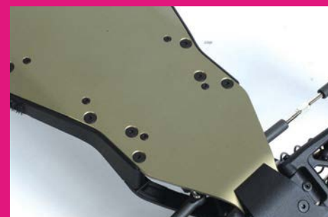
New side rails and more holes in the B6.3 chassis to allow for the updated servo mounts
