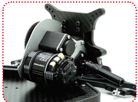
A brushless motor was used for modern-day racing
