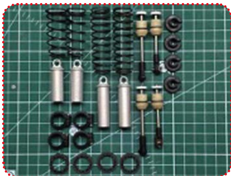
The shock absorber components ready to be built up including re-anodised bodies
