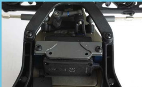
The steering servo mounts are now separate from the rail mouldings
