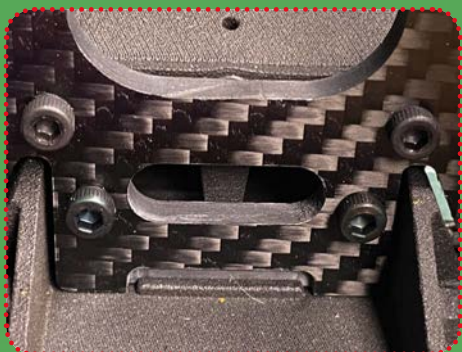
The carbon fibre front shock tower fits inside and bolts through the front bulkhead
