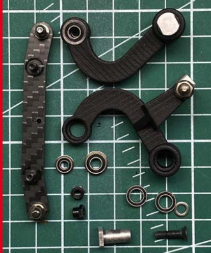
The high-spec package includes a carbon fibre drag link and ball raced steering
