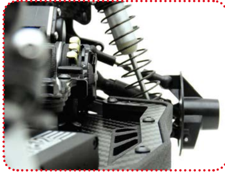
The beautiful printed side rails complete with carbon fibre stiffeners fitted
