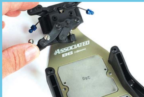
The chassis length markings are now found up front under the updated steering assembly
