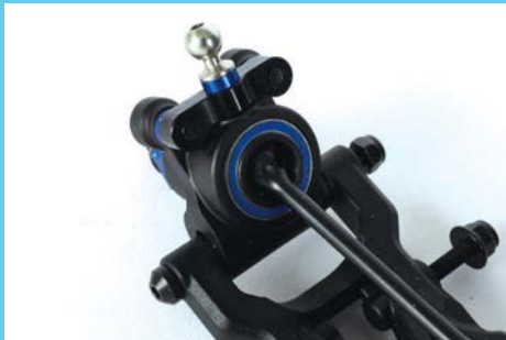
Using the largest possible bearings in the rear hubs ensures strength and durability
