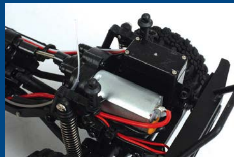
A brushed motor is smoother than a brushless version especially at low speed so is ideal for this application
