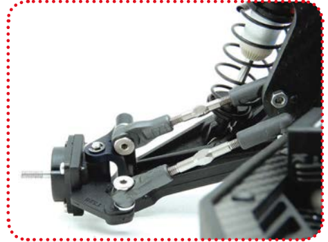
Rose-joints are used on the outboard pivots
