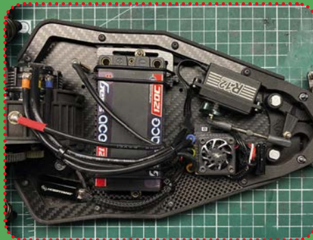
The finished design uses a shorty LiPo and there is plenty of space for the rest of the electronics
