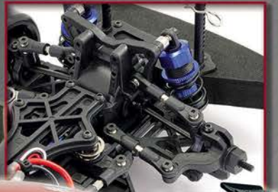
Adjustable big bore oil filled shock absorbers. Below: Adjustable turnbuckles.
