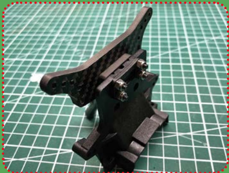
Carbon fibre was used for the rear shock tower
