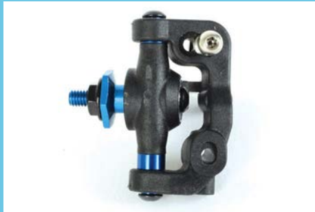
Fine-tuning up front is plentiful with the ability to raise or lower the position of the steering arm in the caster block
