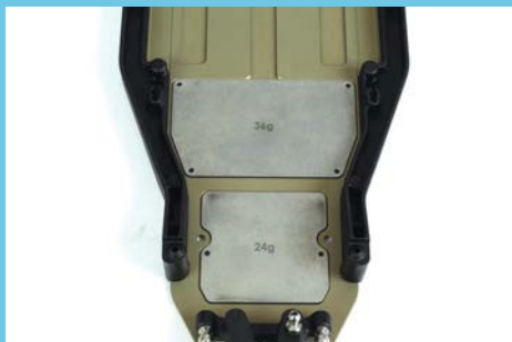
A set of weights sit under the servo and the electronics as found in the B6.2 model
