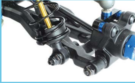
The lower rear shock mounting is secured using a nut for reliability
