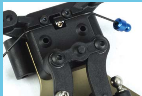
Here you can see the revised bell crank post brace. The moulding now locates into the top plate
