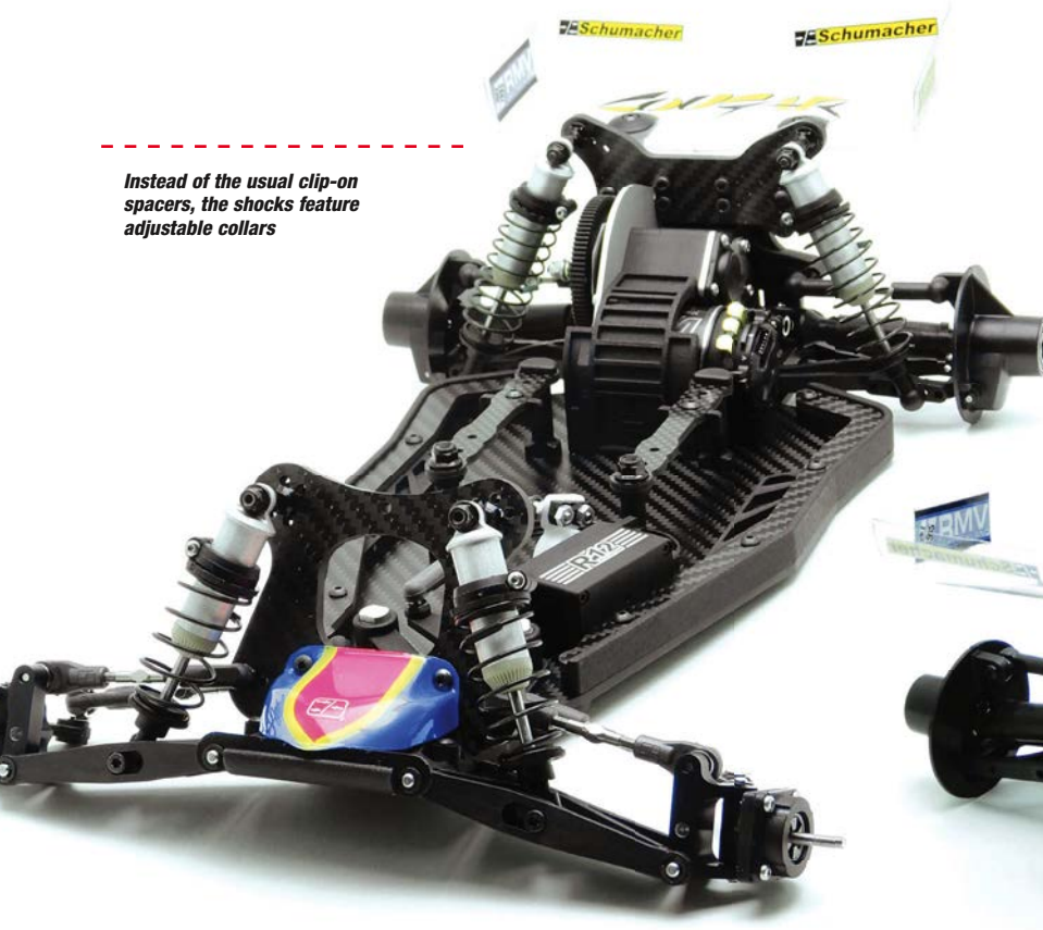
The battery position is very flexible and can be located further rearward if required
