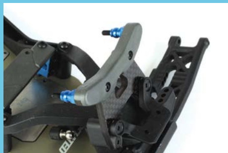
A new moulded protector uses small bolts to secure it to the front shock tower
