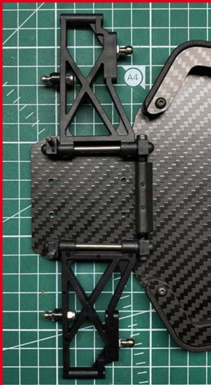
The rear wishbones are original Schumacher Cougar items
