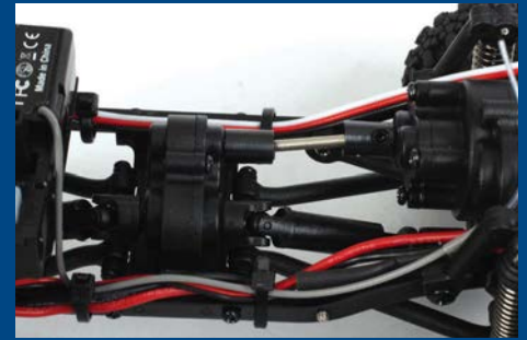
The 'divorced transfer case' allows a single input to be split into two outputs for the front and rear axles
