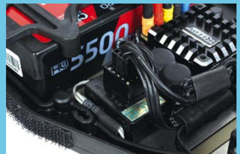
No need to use the aerial tube as we coiled up the wire and secured it with a little heatshrink
