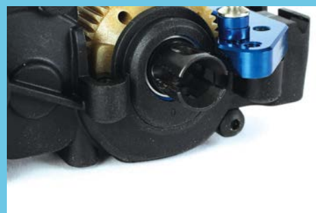
There are four different height positions to choose from for the gear diff
