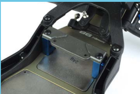
The servo is now secured using new alloy posts that screw to the chassis as well as a moulded top brace
