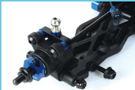
The rear hub design offers lots of tuning potential using spacers to set the ball stud position and the roll centre
