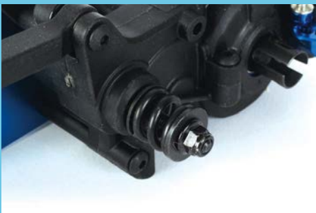
On the other side there is the heavier RC10B74.1 slipper spring
