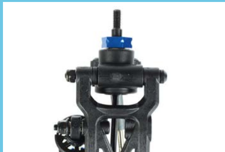
The rear hub controls the wheelbase setting and uses a captured hinge pin design
