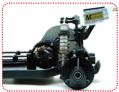
The iconic rear hub design aimed to eliminate dirt getting inside the dished wheels
