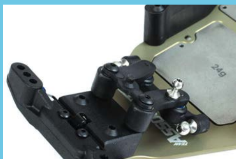
The new steering setup aims to eliminate any excessive play as well as prevent the screws from breaking
