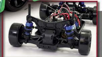
Adjustable big bore oil filled shock absorbers. Below: Adjustable turnbuckles.
