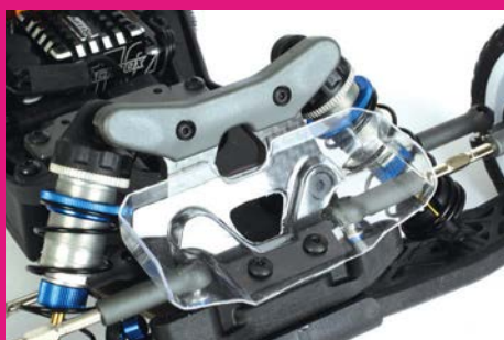
The front wing is trimmed around the holes in the carbon fibre shock tower
