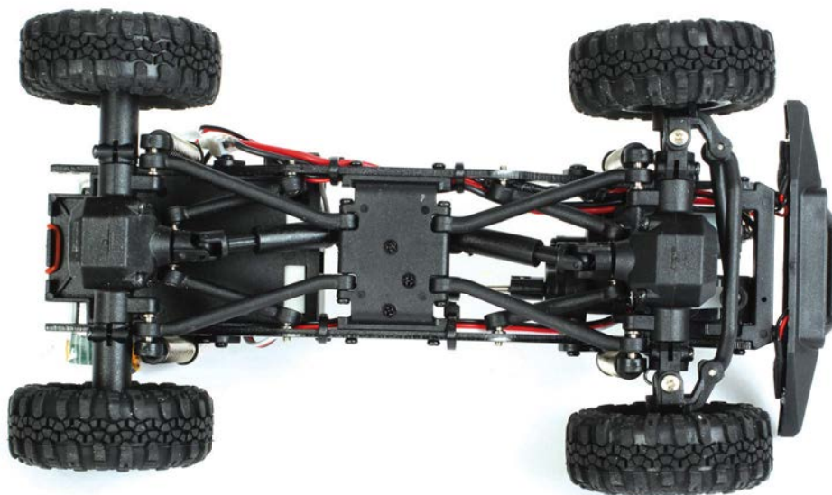
Here you can see the metal vertical chassis rails and 4-link suspension
