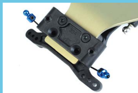
The standard bulkhead is made from plastic, but alloy, steel and brass options are popular for tuning
