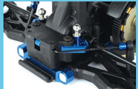
Anti-roll bars are included both front and rear to suit high-traction race surfaces
