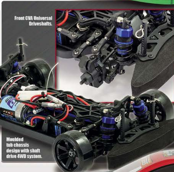
Adjustable big bore oil filled shock absorbers. Below: Adjustable turnbuckles.
