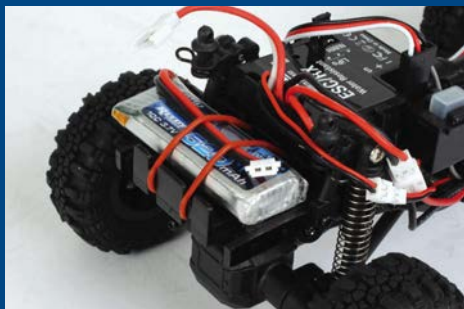
To ensure great rear traction the electronics including the LiPo battery are positioned over the rear axle
