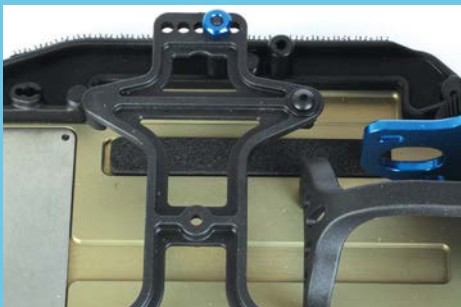
With the Laydown gearbox the battery location options are quite limited
