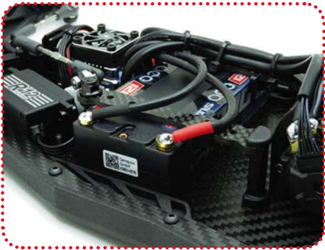
The battery position is very flexible and can be located further rearward if required
