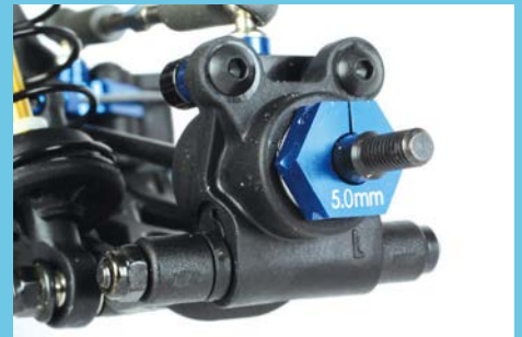
5mm offset hexes are used both front and rear
