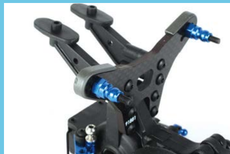
A new rear shock tower protector sits on either side
