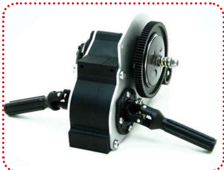
The gearbox has been tweaked with an updated slipper clutch
