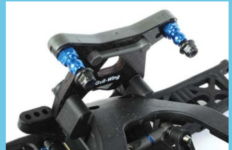
The front tower has been tweaked for the B6.3 with a revised shape and new shock positions
