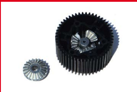
The diff is of the planetary geared-type design
