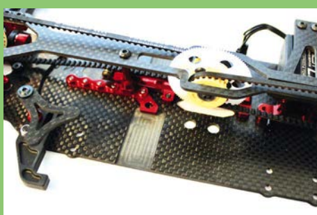
High quality carbon fibre is used for the chassis, top deck, shock towers and more
