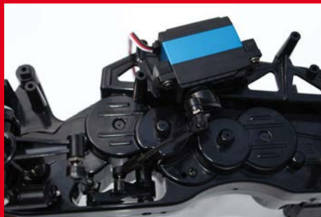
The Carson steering servo hangs off the side of the GF-01CB chassis
