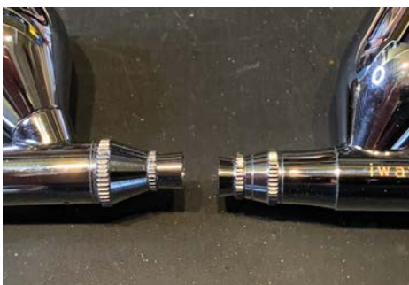
Here you can see how the shape of two airbrush nozzles differ
