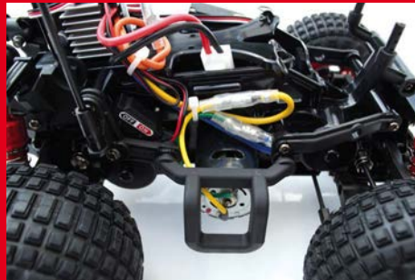
A neat moulding protects the end of the Mabuchi RS-540SH brushed motor
