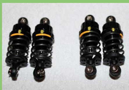
The "V4 Short Big Bore" shocks. All four are of the same spec and were built with zero rebound
