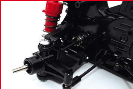
The steering linkages use adjustable threaded rods. Ensure that these are the correct length for the best handling
