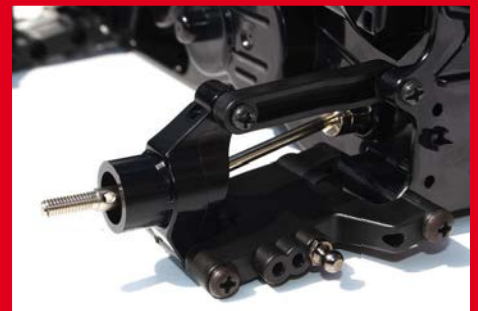
Dogbone driveshafts are used both at the front and rear
