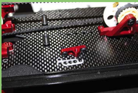
One of the lightened shims used on the bulkheads
