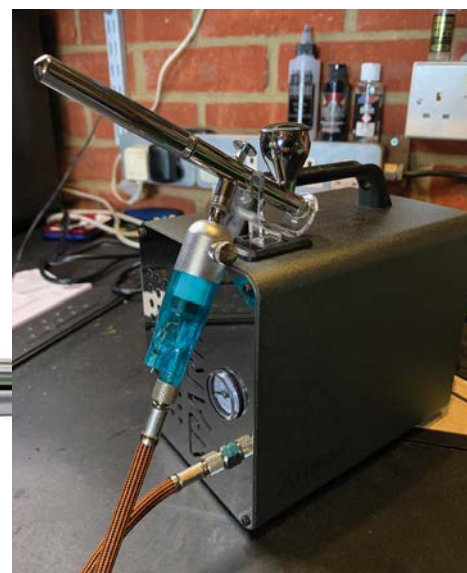
The Sparmax Arism Viz compressor with their Magic Bullet Plus Valve installed
