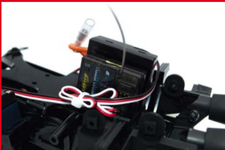
The receiver is a Carson Reflex Wheel 3 Pro 2.4GHz model
