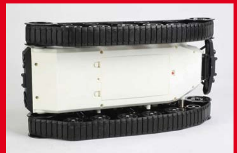
The underside is smooth and with lots of clearance allows the Buzzsaw to be used in rough conditions
