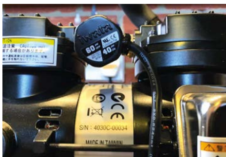
The Iwata compressor has a built-in auto pressure switch
