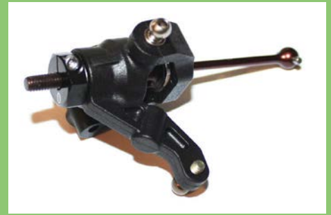
The front hub assembly ready to go on to the car. The alloy bushings ensure no binding in the movement
