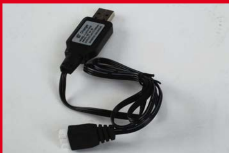
Like so many smaller-sized RTR machines, the Buzzsaw comes with a USB-type charging lead
