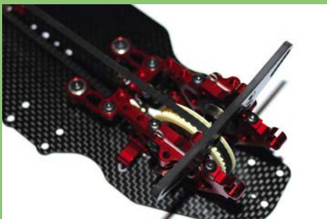
The steering assembly, once fitted into position moves very freely on bearings
