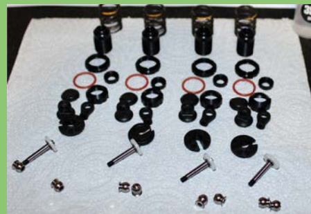
All of the components for a complete set of four V4 big bore shocks
