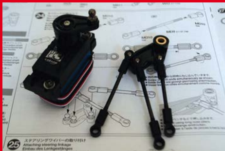
The Carson Reflex CS3 servo for the steering and the bell crank it connects to
