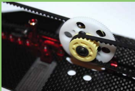
Note the machined section of the carbon fibre chassis to allow the motor to sit as low as possible
