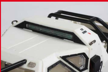
On the top of the body is an LED light strip that is very bright when turned on
