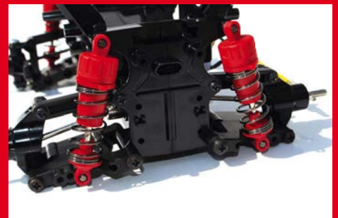
With the rear shocks in position, located on by ball joints top and bottom
