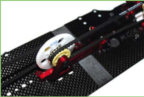
With the layshaft, diff and spool in place, it is just the top deck to fit
