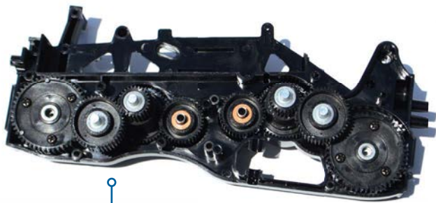
The entire transmission sits on a mix of brass and plastic bushings
