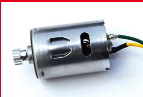
The kit Mabuchi RS-540SH brushed motor is more than powerful enough for the Comical model
