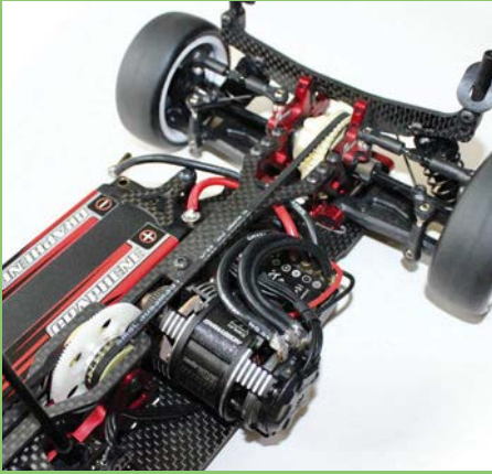
The Hobbywing 13.5T motor is controlled by an Orca OE101, perfect for blinky racing
