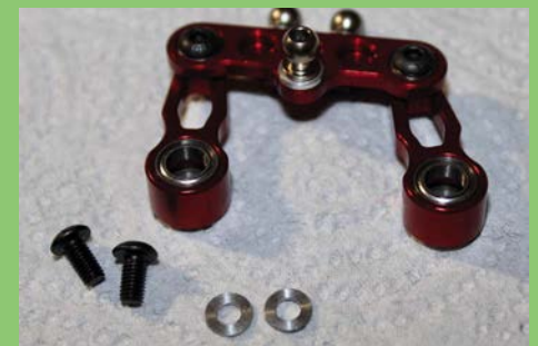
Capricorn supplies alloy steering arms in the kit, compared to others who include plastic as standard with alloy as an option
