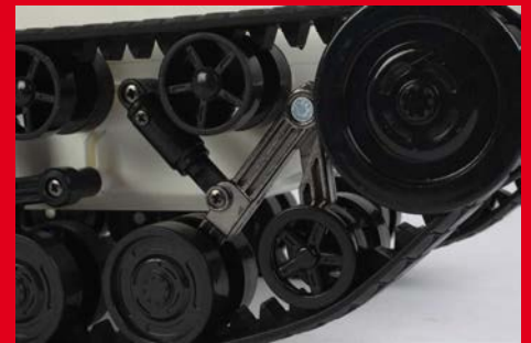
The design allows the tension on the tracks to automatically adjust to the surface
