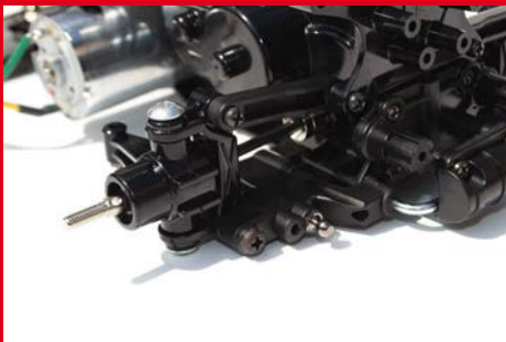
Fixed length moulded linkages means a fast build with perfect geometry out of the box
