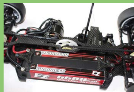
An EZ Power 6600mAh Graphene LiPo battery was used for our testing
