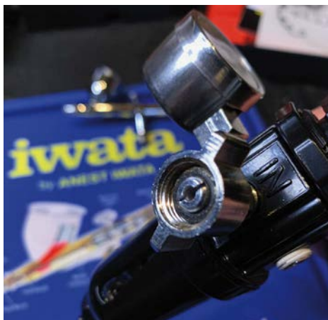
The 0-ring seal in the fitting for the Iwata air pressure regulator and moisture trap
