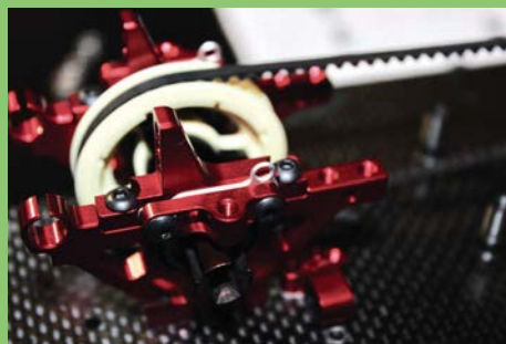
With the shim in place, you can still see the locator for easy removal
