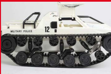
Here you can see the dampers that control the movement of the tracks
