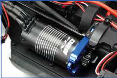
The sensorless brushless motor is a 4-pole design and rated at 2000Kv
