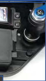
The 2.4GHz receiver sits inside a moulded protective box
