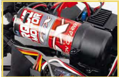
The reduction gearbox (red) offers improved torque and benefits low-speed driving
