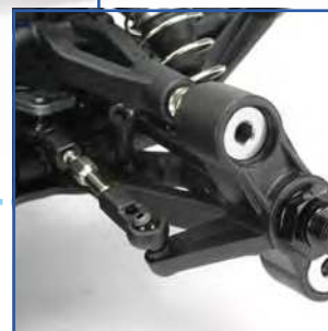
Race-inspired pivot-ball suspension up front
