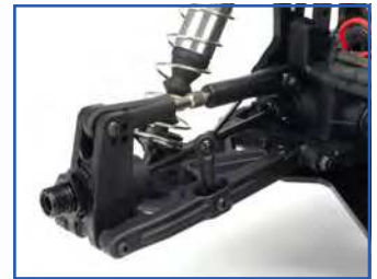
Adjustable linkages and a choice of roll centres are just some of the tuning options
