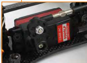
Schumacher supplied a Core RC 9009LP low-profile servo which was perfect
