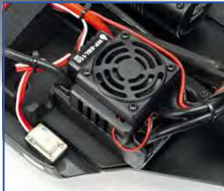
The Hobbywing 150A brushless speed controller is a proven unit
