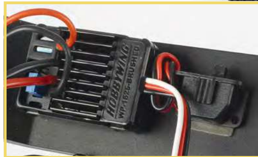
The speed control is a waterproof Hobbywing 25A brushed model
