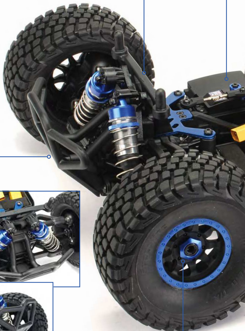
The front bumper features a skid design to help assist the DR8 over obstacles
