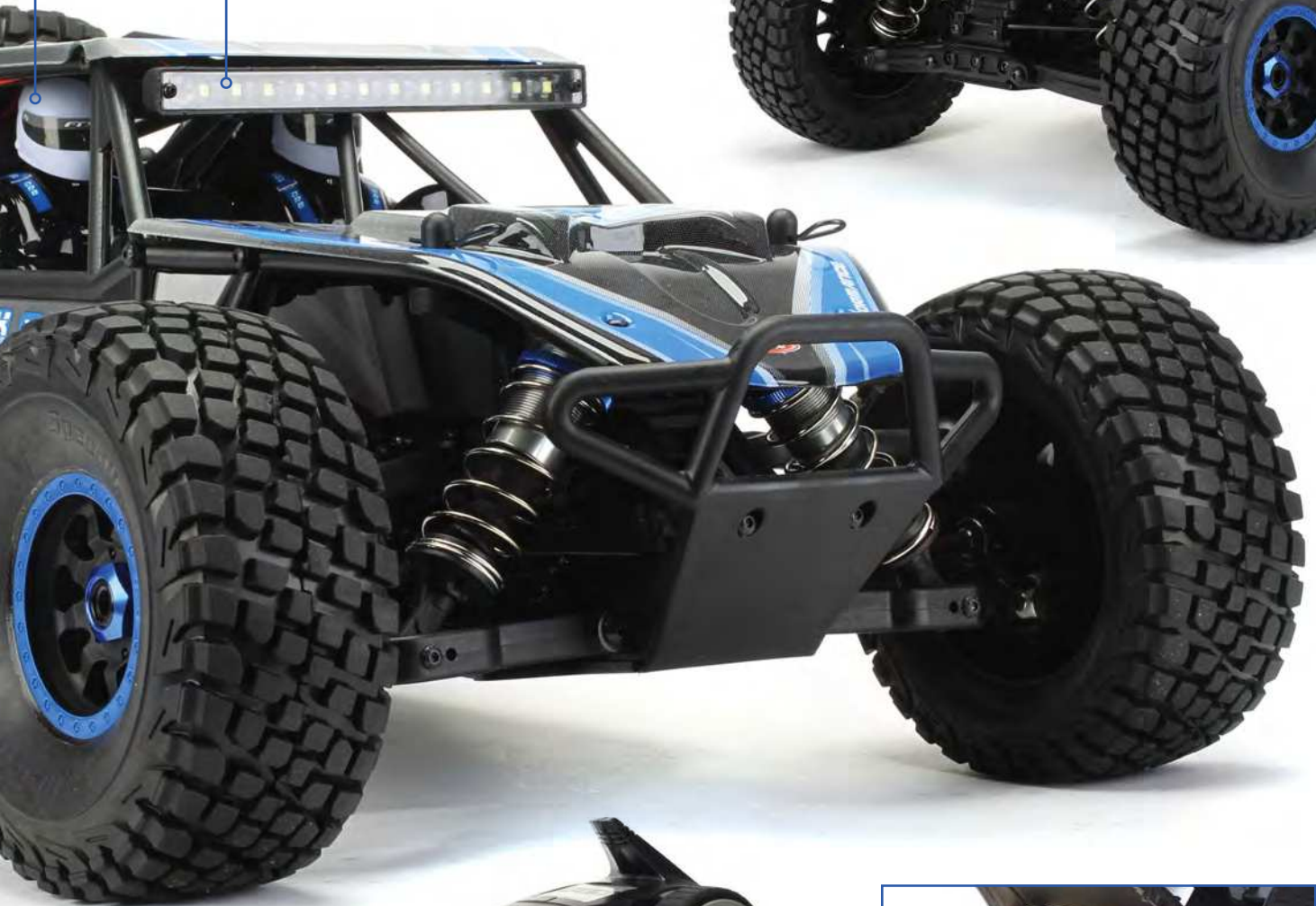
There are LED light bars fitted both front and rear
