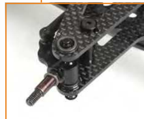
Carbon fibre upper and lower wishbones with an alloy steering block. The ride height is set using shims below the steering block
