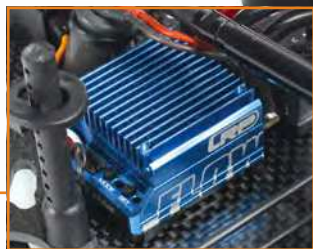
The venerable LRP Flow Works Team sensored brushless speed controller
