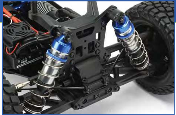
Big bore aluminium threaded oil-filled shock absorbers are design to take big hits
