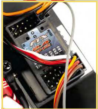
Part of the included radio system is the 2.4GHz 4-channel receiver
