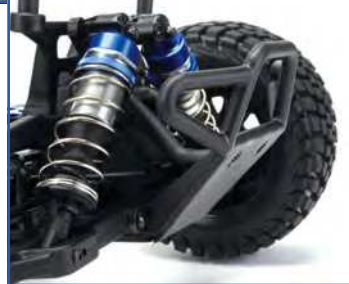
The front bumper features a skid design to help assist the DR8 over obstacles
