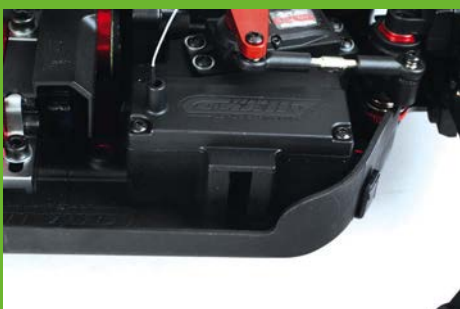
The Variprop 2.4GHz receiver is well protected by a moulded box
