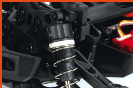
A nice alloy adjuster is fitted to each of the moulded shock bodies
