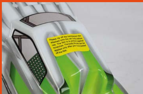
The protective film has to be removed off the body before applying the decals
