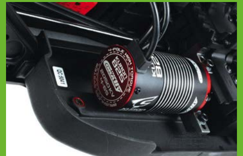
The motor of choice is one straight from the Corally stable in the form of a Kuron 825 4-Pole 2050kV model
