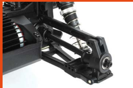
Moulded plastic driveshafts are used throughout
