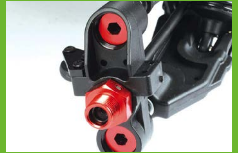
Corally's red theme continues with the pivot-ball front suspension components
