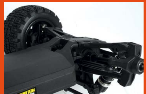
The design allows the main chassis to sit up higher than the front and rear suspension/gearbox modules
