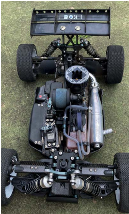
Settings include 10k (F)/15k (C)/5k (R) diff oils, 550cst (F)/500cst (R) shock oils, MIP shock pistons, kit springs and a Protek clutch
