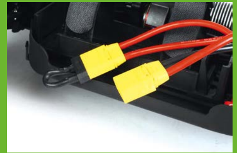
With the jumper cable in place you can hook up a single 6S LiPo rather than a pair of 3S packs
