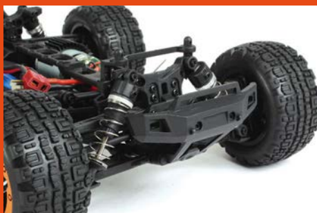
A wide bumper sits ahead of the front shocks to offer protection
