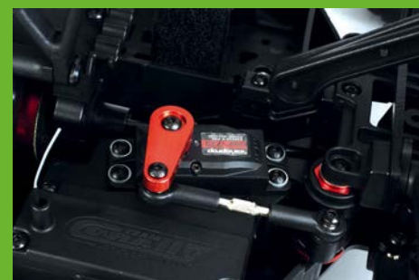
The steering servo is metal-g geared, is rated at 25kg of torque and performed well during testing
