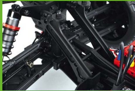
The gearbox and wing get some serious bracing at the rear of the chassis
