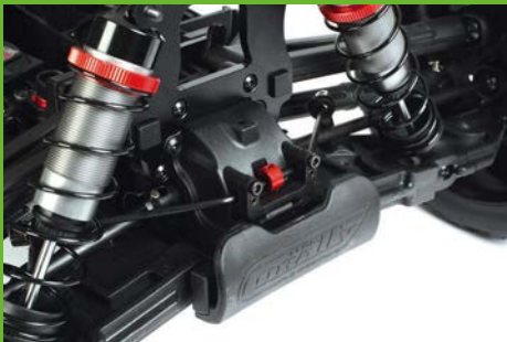
A minimalist front bumper gives some protection to the gearbox
