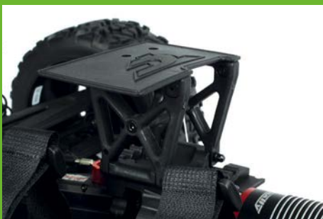
The aforementioned central body support also acts as handle when the shell is removed
