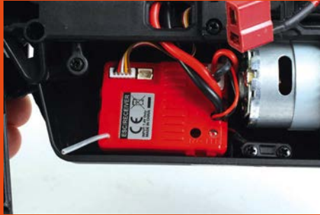
The speed controller and receiver are incorporated into a single unit
