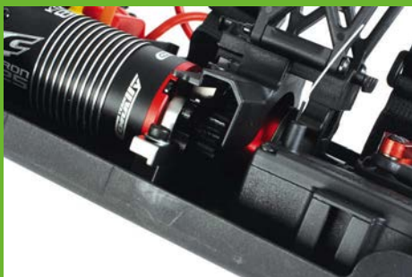
A neat moulDED cover ensures fingers or other small items can get into the spur and pinion area
