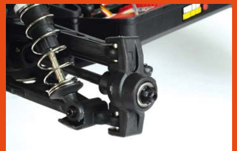
Bearings, like you see here inside the front upright, feature throughout the model
