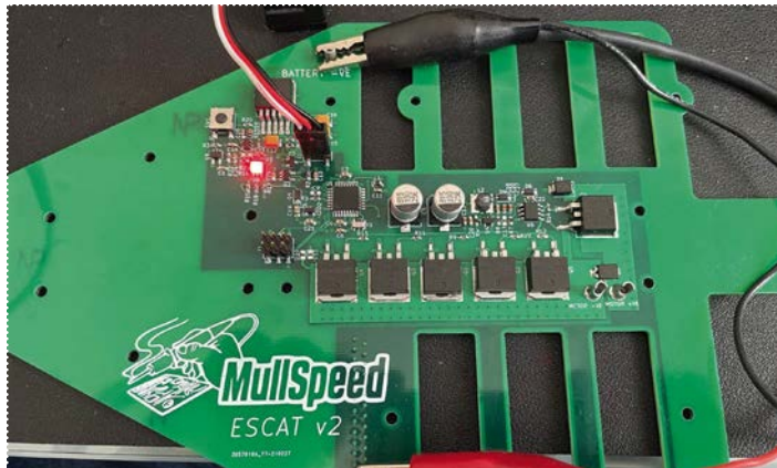
Testing the speed controller by connecting power directly to the posts
