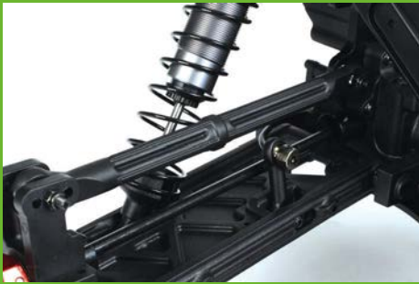
The use of moulded fixed length linkages will always divide readers but its a great choice in our opinion
