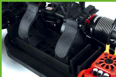
The battery compartment has been designed to be as flexible as possible to suit a range of setups
