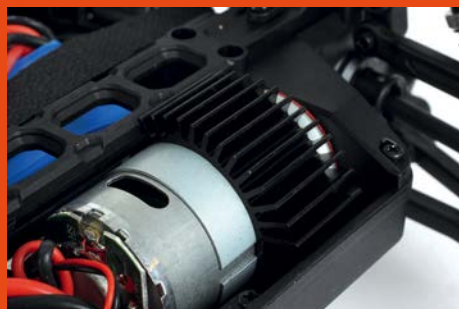
A clip-on alloy heatsink will help keep that motor nice and cool in long runs
