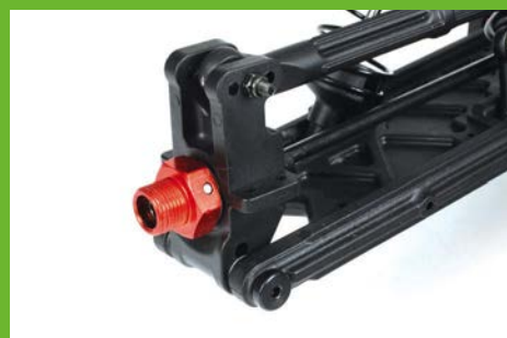
Threaded outer hinge pins secure the rear hubs in place no small E-clips to fly off
