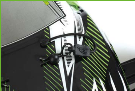
A retaining system on all four body clips means searching for missing ones are a thing of the past
