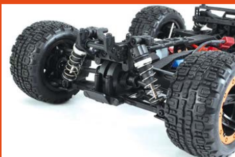
This image of rear of the Tracer Truggy shows the body mounts bolted to the shock tower and wide tyres
