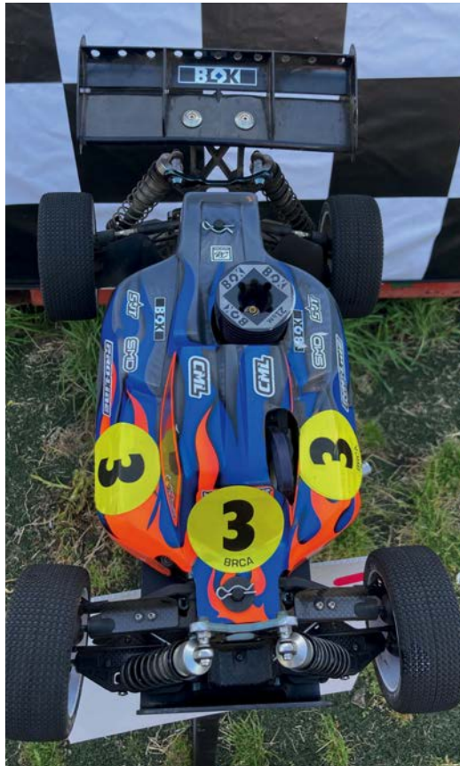
The winning buggy shod with Pro-Line Sidelock tyres, powered by a Blok engine and running OptiPower nitro fuel
