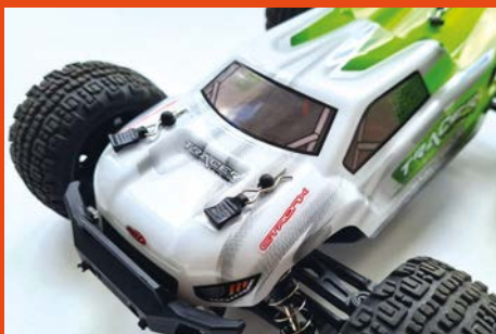
Neat moulded tabs on the body clips ease removal
