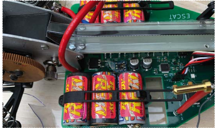
By using the chassis space the speed controller components are well spread out
