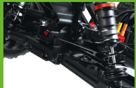
Anti-roll bars front and rear will prevent excessive chassis roll at speed in the corners
