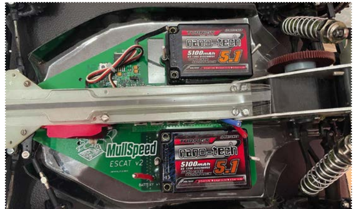
The ESCAT v2 can accept LiPo power in the form of saddle packs
