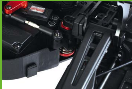
There is plenty of adjustability to be had with the caster angle and servo saver setting as just two examples
